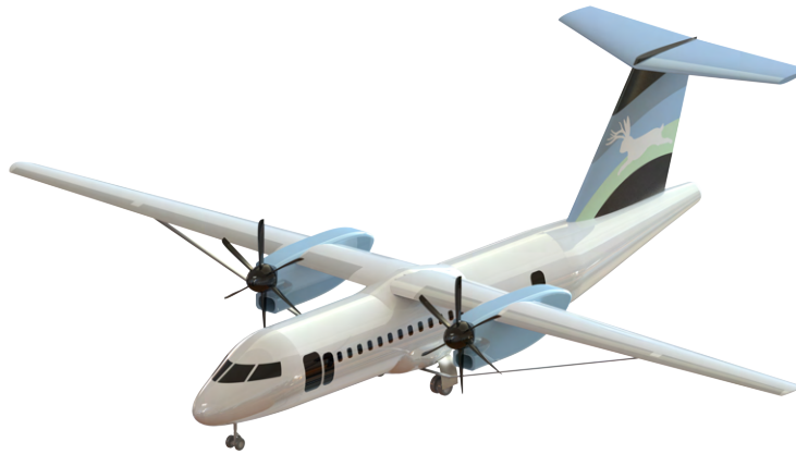
Fig. 10 Final Configuration with Truss-Braced Wing
