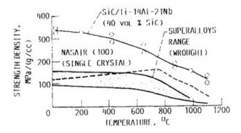
Figure 15: Physical property comparison of MMCs and traditional nickel-based superalloys [22]
