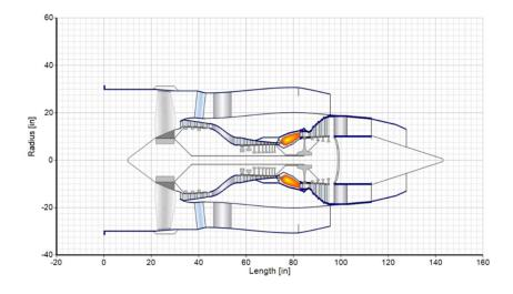
Figure 18: Detailed cross-section of the Dream Stream turbofan
