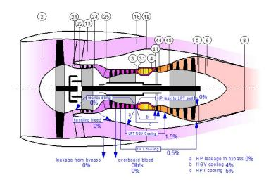
Figure 17: Conceptual cross section highlighting each station number
