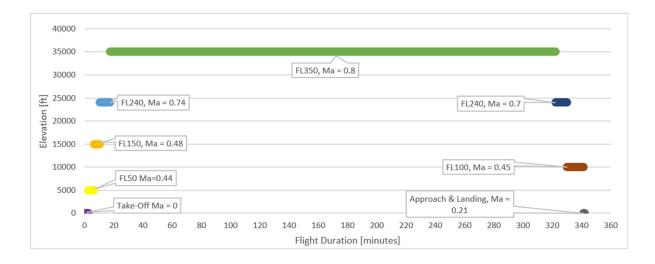
Figure 24: Plot of the approximated mission profile of a Boeing 737-800 aircraft
