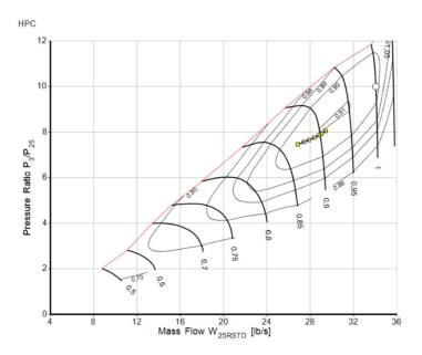
Figure 23: HPC off-design operating line
