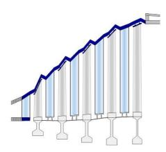
Figure 5: LPT design with additional stage
