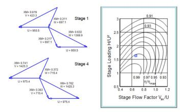
Figure 20: Low pressure turbine velocity diagrams and Smith chart
