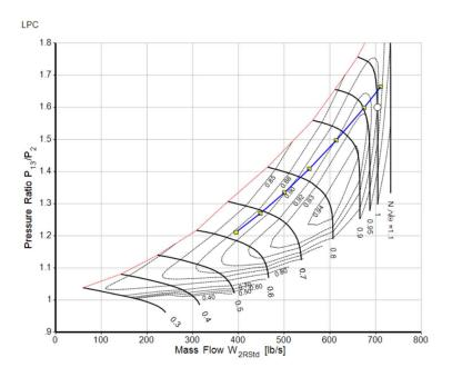
Figure 21: Fan off-design operating line
