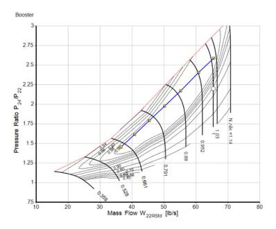
Figure 22: Booster off-design operating line
