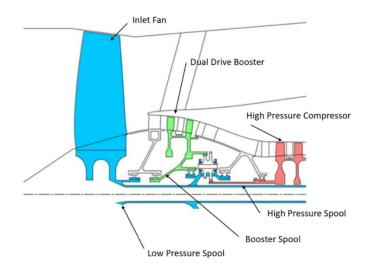
Figure 1: Dual drive booster spool schematic [11]
