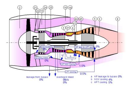
Figure 2: Generic cross section of an unmixed turbofan with station numbers in GasTurb14
