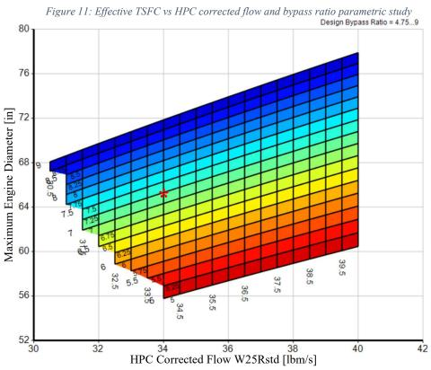
Figure 12: Maximum engine diameter vs HPC corrected flow and bypass ratio parametric study
