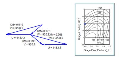
Figure 19: High pressure turbine velocity diagrams and Smith chart
