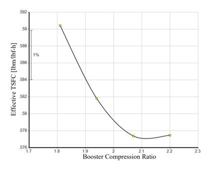
Figure 10: Effective TSFC vs booster compression ratio parametric study
