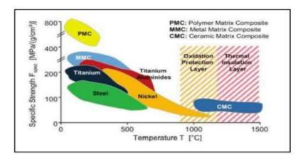
Figure 13: Comparison of composite and traditional turbofan materials [17]
