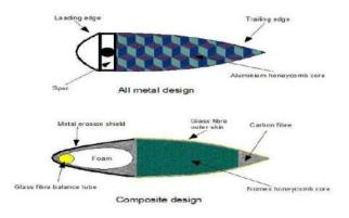
Figure 14: Inlet fan blade cross section comparing metal and composite designs [17]
