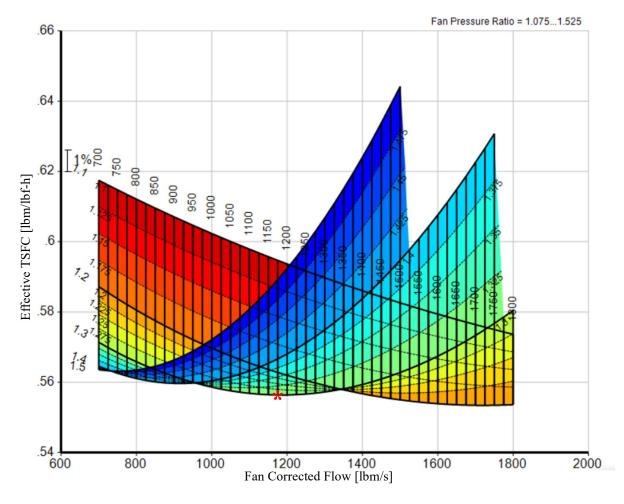
Figure 9: Fan corrected flow and fan pressure ratio parametric study
