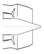
Figure 6: Mixed nozzle turbofan design
