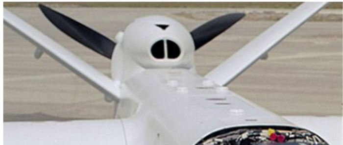
Figure 4.12: Inlet Cross-Section of General Atomic MQ-9 Reaper [21]
