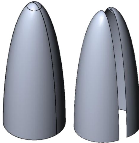
Figure 4.9: Clam shell release fairing design
