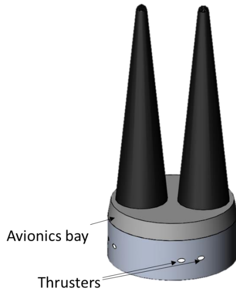
Figure 4.8: Post-Boost Vehicle Design
