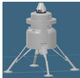
(b) Second Configuration Proposal From top to bottom; crew module, service module with cargo compartments on the sides.
