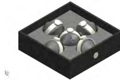
Figure 10.2: AA Configuration with Five CMGs
