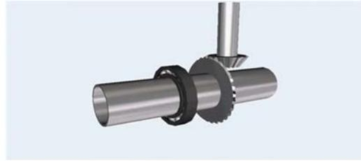
Figure 7.3: Bevel Gear Connection to Propeller Shaft
