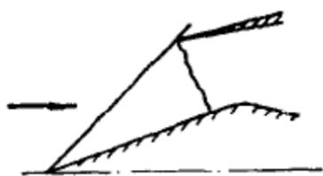
Figure 5.2 external compression inlet
