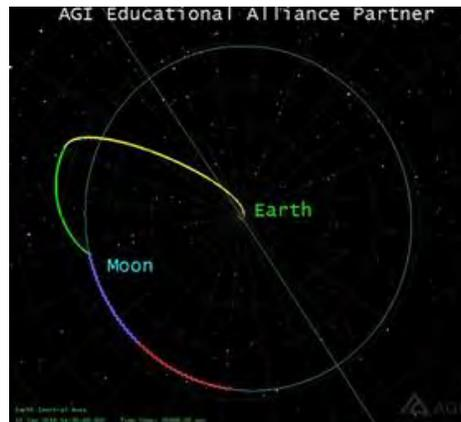
**Figure 48: Model of the bi-elliptic transfer in STK.** The STK model of the bi-elliptic transfer displays the trajectory of the Orbiter on its way to the Moon. The middle burn is located where the yellow and green portions of the trajectory intersect.
