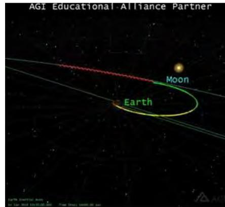
**Figure 47: Model of the Hohmann transfer in STK.** The STK model of the Hohmann transfer displays the trajectory of the Orbiter on its way to the Moon. Once reaching the Moon, the Orbiter goes into a polar orbit to go over the desired craters.
