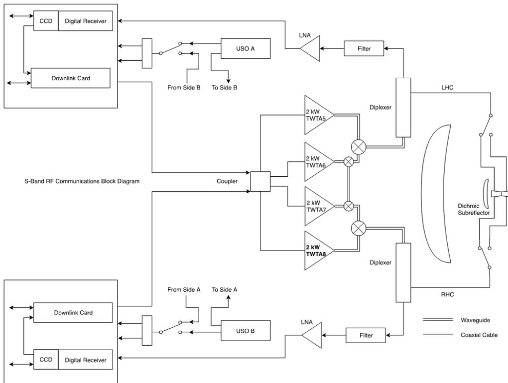
Figure 34: HGAS and LGH Block Diagram
