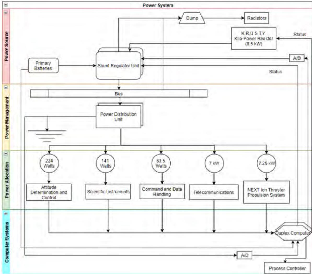
Figure 26: Power System Block Diagram
