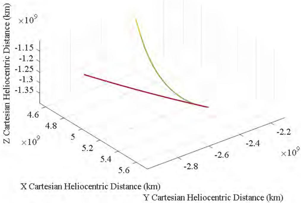
**Figure 16: Enlarged Off-Axis View of Burn Phase (Pluto Orbit = Red, Cruise = Yellow, Burn = Green)**
