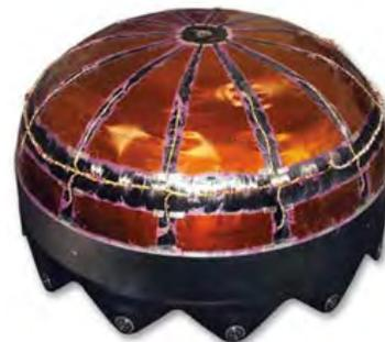
**Figure 21: Cobham Xenon Tank [72]**
