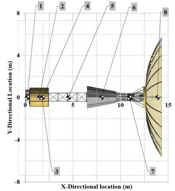
Figure 35: XY View of CM Locations of PROSERPINE (Scale 1:200)
