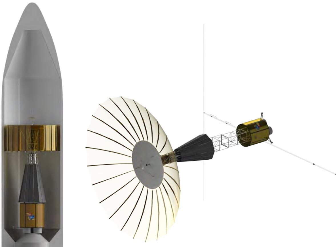
**Figure 1: Rendering of PROSERPINE within Atlas V 552 and Deployed**
