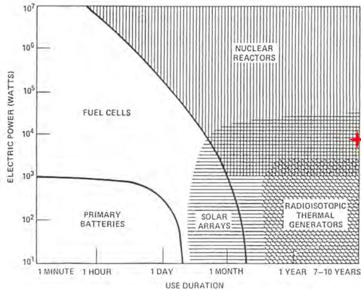
**Figure 23: Power System Design Selection [49]**
