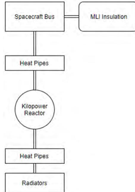
**Figure 27: Thermal Control System Block Diagram**
