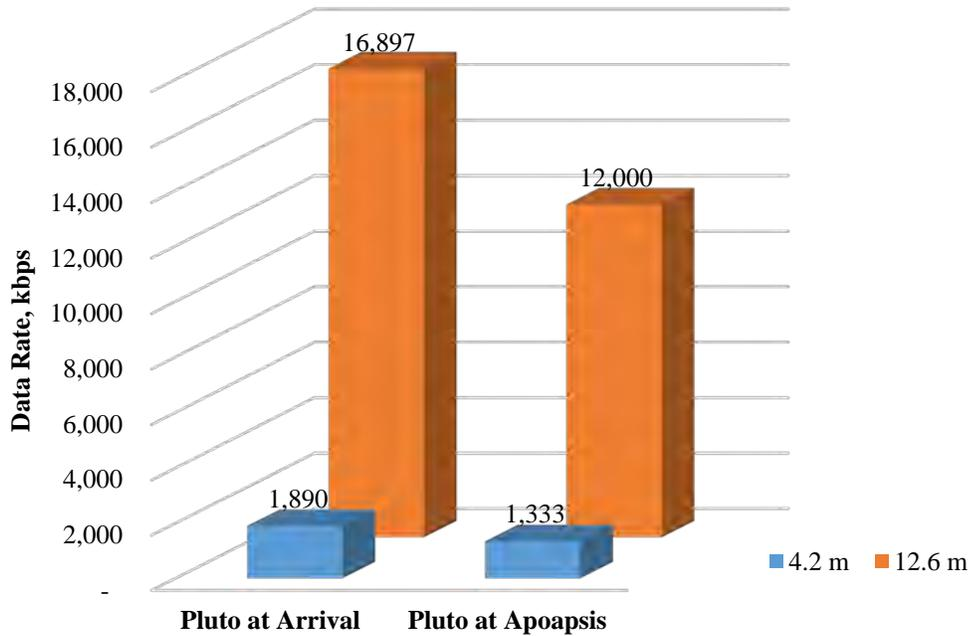
Figure 32: X-Band Transmitting Data Rates for Each Antenna Diameter at Arrival at Pluto and at Apoapsis of Pluto, 6000W at 3 dB Margin
