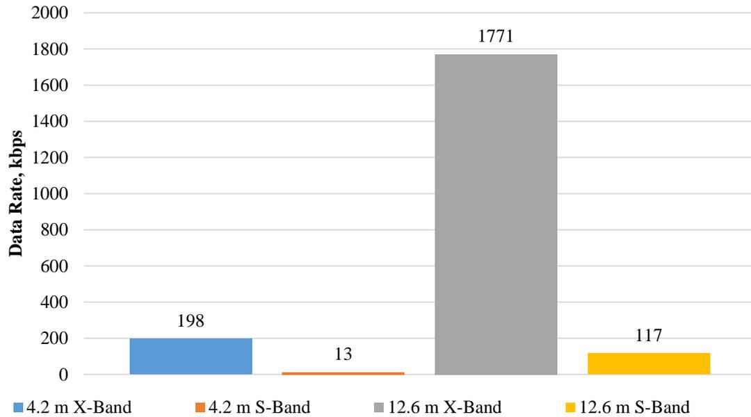
**Figure 30: Transit Science and Engineering Downlink Capabilities with 700 W Transmission to DAEP 34-m Antenna Arrays**
