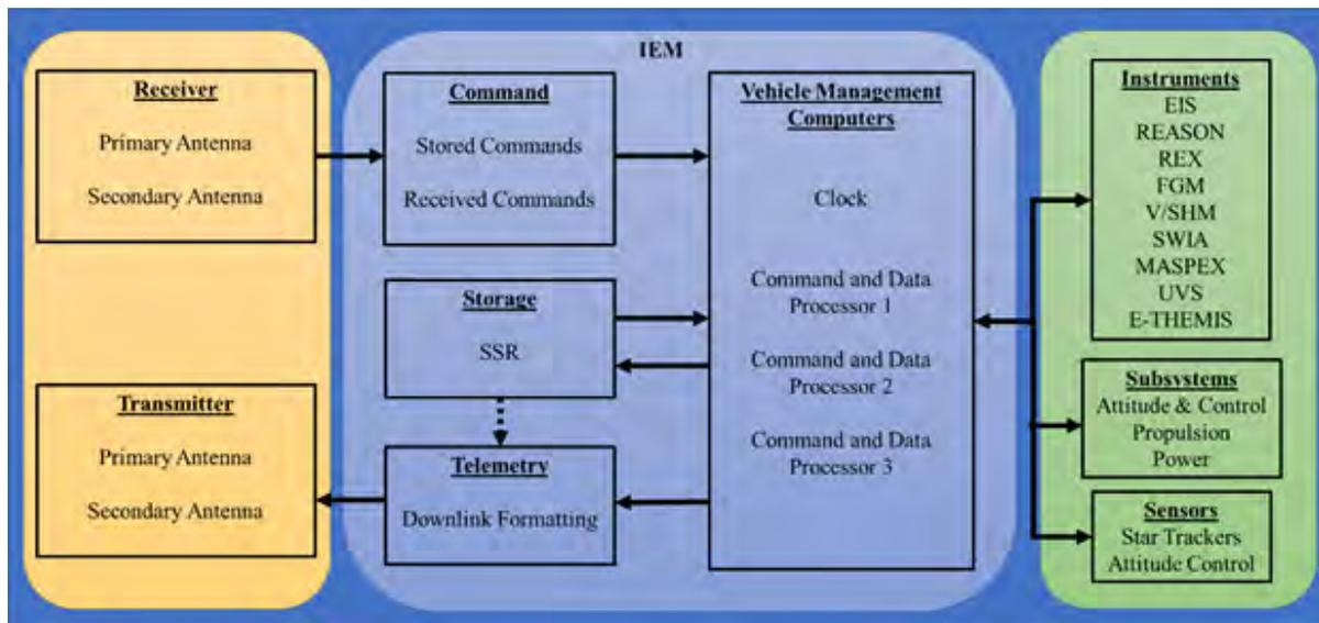
**Figure 28: C&DH Block Diagram**
