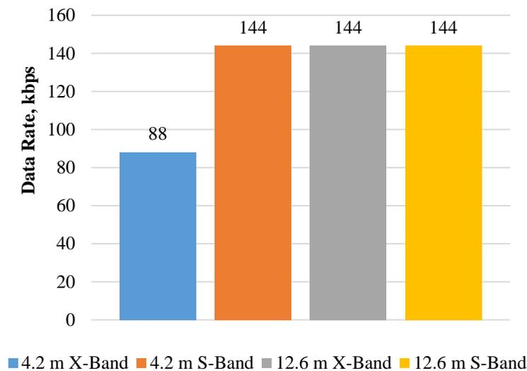
**Figure 29: Command and Control Uplink Capabilities with DAEP 34-m Antenna Arrays**
