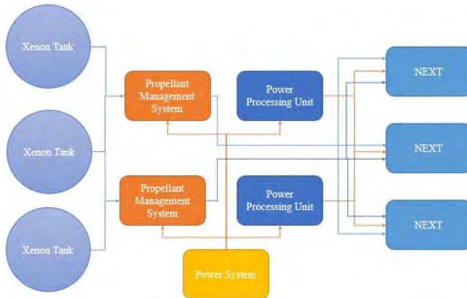
**Figure 22: Propulsion System Power Diagram**
