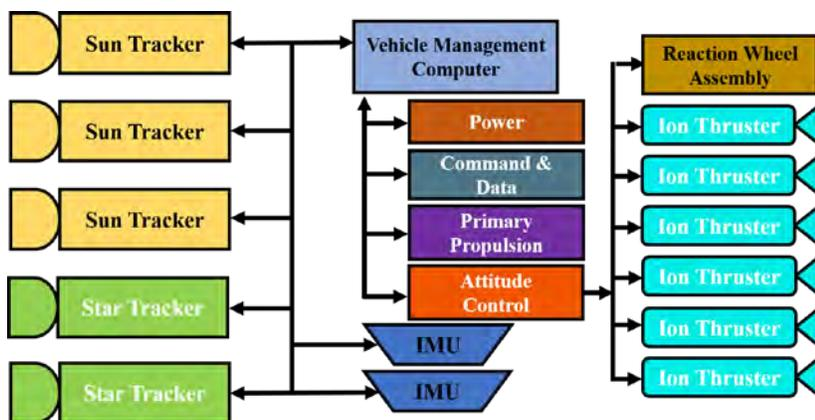
**Figure 39: Block Diagram for AD&CS Integration**
