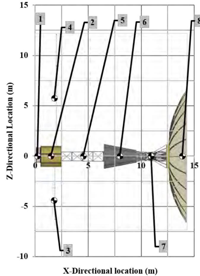
Figure 36: XZ View of CM Locations of PROSERPINE (Scale 1:200)
