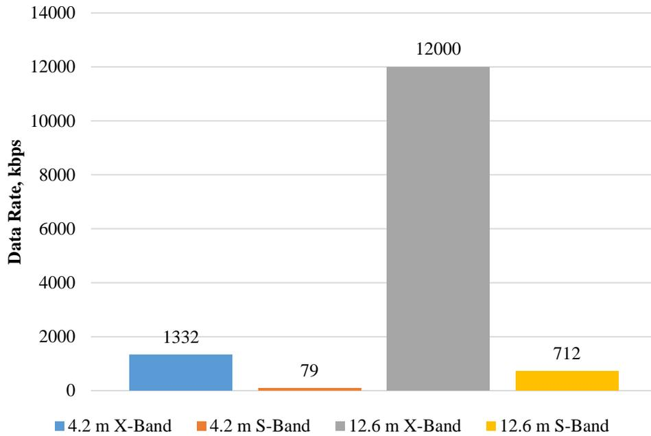
**Figure 31: Orbiting Science and Engineering Downlink Capabilities with 6000 W Transmission at 50 AU to DAEP 34-m Antenna Arrays**
