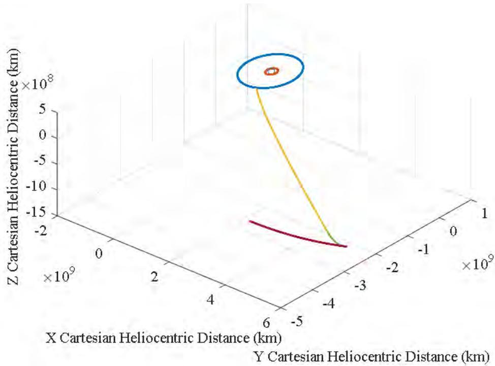
**Figure 15: Off-Axis View of Trajectory from Jupiter to Pluto (Sun = Light Blue, Earth Orbit = Orange, Jupiter Orbit = Dark Blue, Pluto Orbit = Red, Cruise = Yellow, Burn = Green)**
