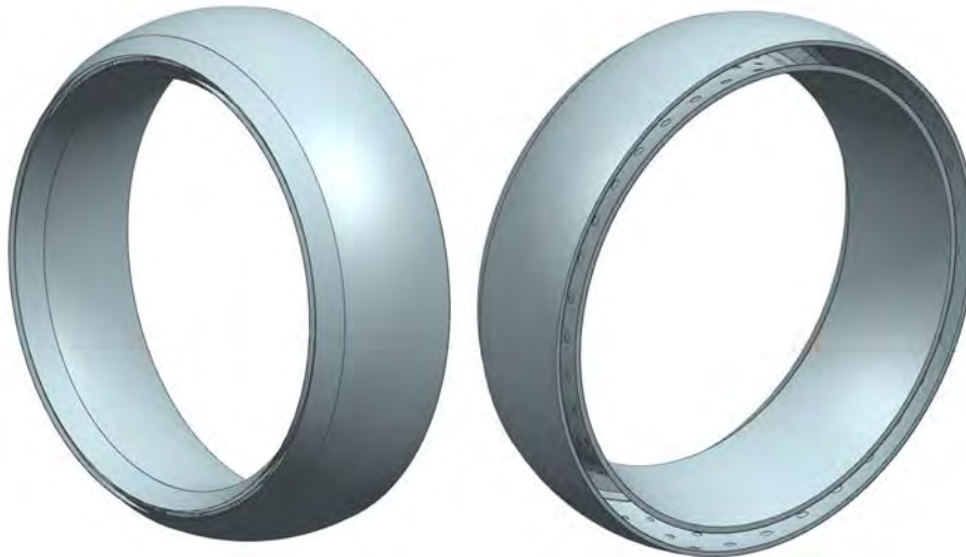
Figure 34: 3D model of combustor chamber, front view (left) and back view (right)
