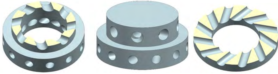
Figure 35: Primary swirler (left), whole swirler (middle), secondary swirler (right)
