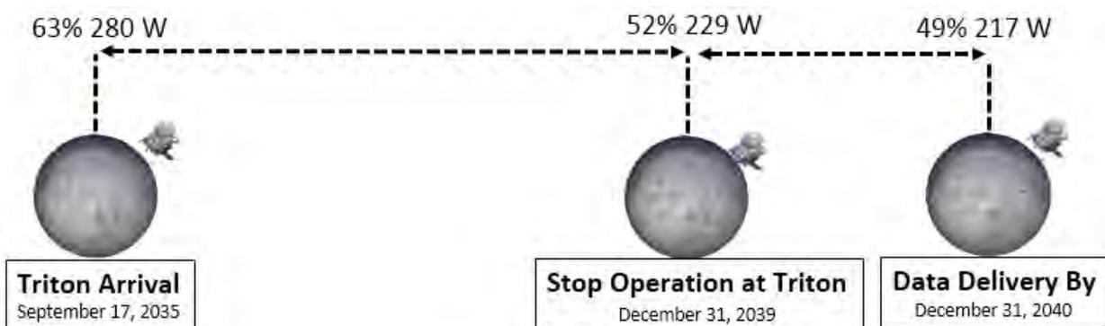
**Figure 10.0-3** Spacecraft Operations Power Degradation from BOL to EOL
