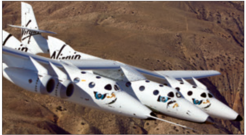
The WhiteKnightTwo carrier aircraft, with SpaceShipTwo, made its first long-distance captive-carry flight in October.
