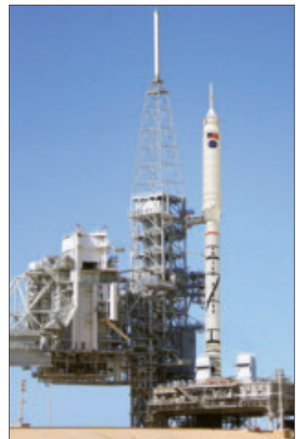
The first flight test of NASA's Ares I-X test vehicle provided important data on ascent loads, vehicle control, separation, and first-stage reentry dynamics.
