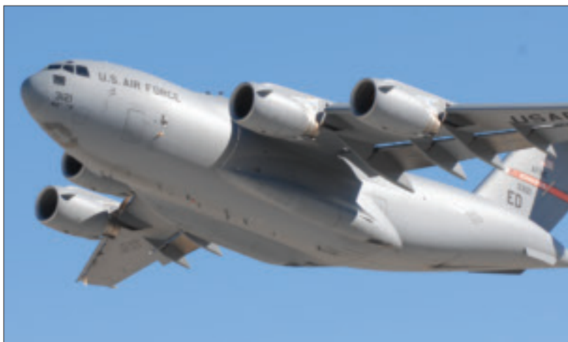
A C-17 Globemaster III takes off August 27 on a flight test to examine how it performs with different combinations of biofuels. The aircraft is powered by 50% JP-8, 25% by hydro-treated renewable jet fuel, and 25% by a Fischer-Tropsch fuel. The 418th Flight Test Squadron conducts flight tests during the week using different combinations of regular JP-8 and the HRJ. Air Force photo by Kenji Thuloweit.
