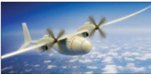
The hydrogen-powered Phantom Eye can stay aloft for four days with a 450-lb payload
