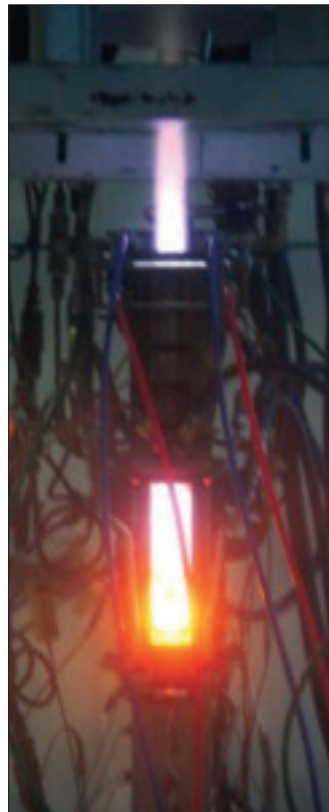
A model scramjet at the University of Virginia uses Stanford tunable diode laser sensors for monitoring the temperature and degree of combustion completeness in the combustor exhaust.
