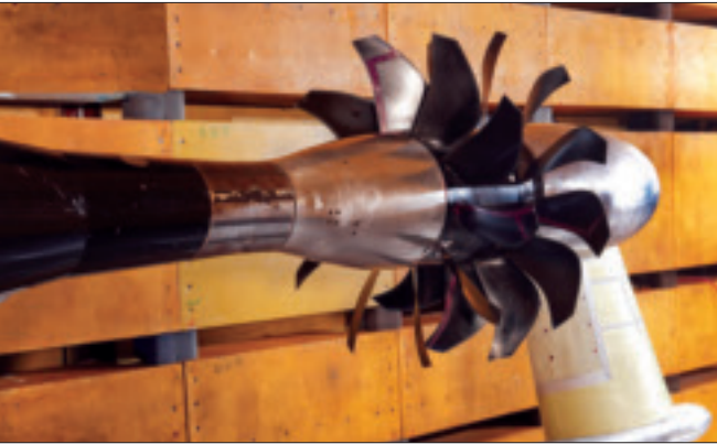
NASA Glenn's wind tunnels are enabling the current NASA/GE collaborative testing of counterrotating fan-blade systems for open-rotor jet engine designs.
