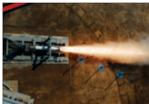
An ASMAT horizontal RATO motor characterization test is conducted at NASA Marshall.
