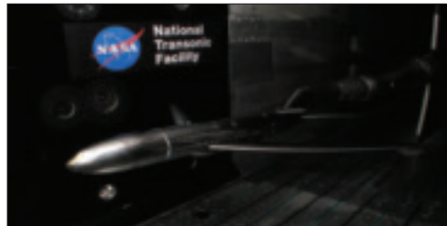
Active damping is used on the wind tunnel sting to help increase data quality.
