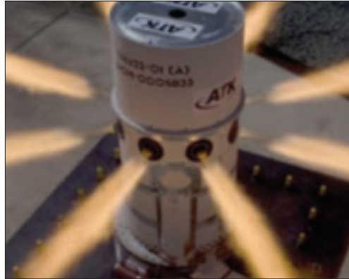
The Orion launch abort system and attitude control motor, both manufactured by ATK, undergo static testing.
