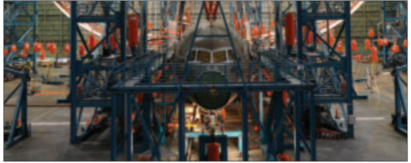
Boeing engineers bent the wings of a 787 ground-test airplane until the load was more than one-and-a-half times anything the jet will experience in service.
