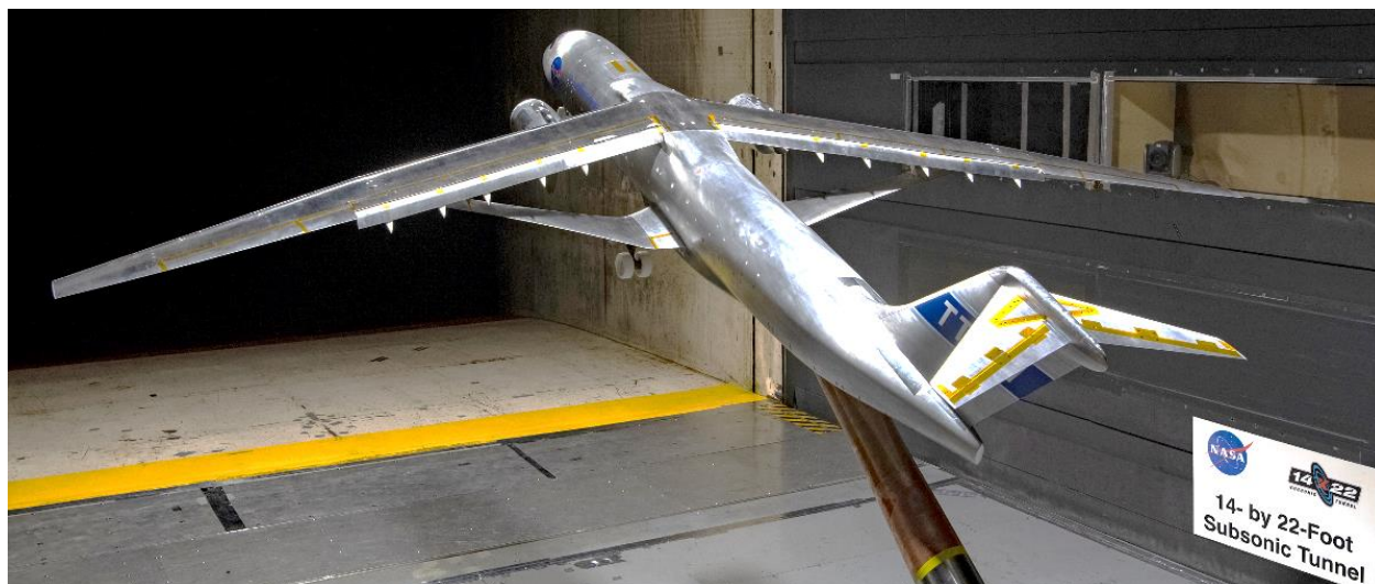
Figure 13. TTBW Low-Speed Test in the NASA LaRC 14- by 22-Foot Subsonic Tunnel
