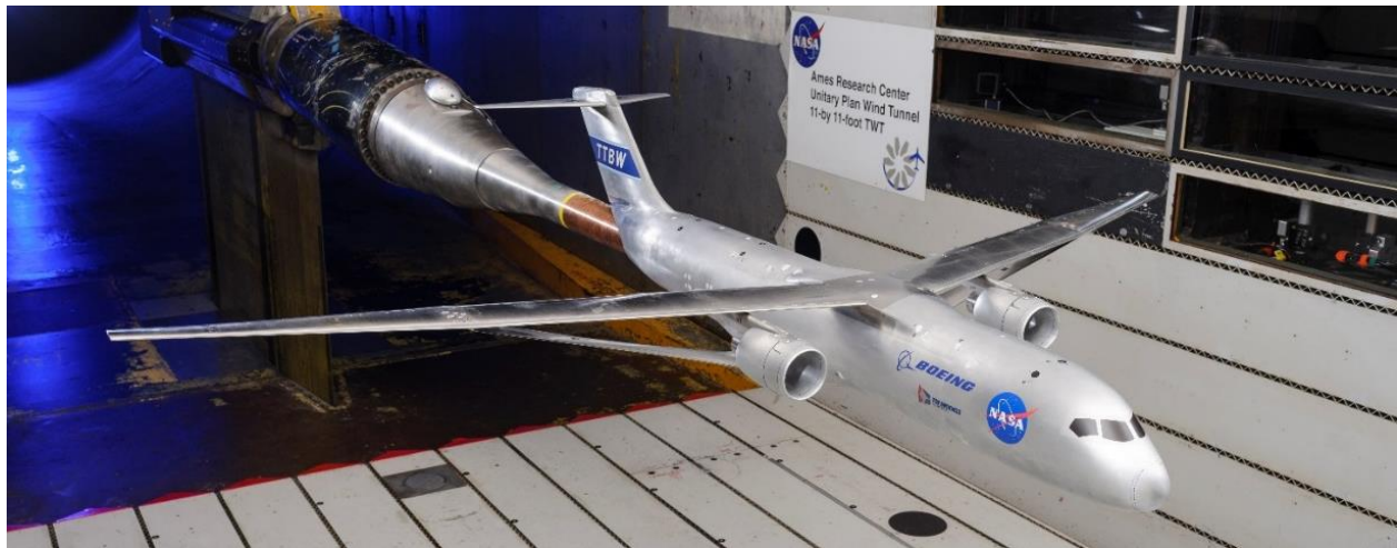
Figure 8. M=0.80 TTBW Configuration in the NASA Ames 11-Foot TWT
