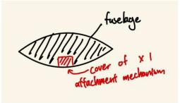
Answer: This would not be allowed or would require cover or door to conceal the mechanism for M1 and at the start of the GM. In this example with the release mechanism flush with the outside of the fuselage, the cover or door may be permanently removed for M2 and M3 and after installing the release mechanism during the GM.
