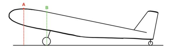
Answer: The rules clearly state "while resting on its landing gear", which means ALL gear and contact points (in the case a rear tail skid is used in place of a wheel). In the example provided, the maximum height of the blocks cannot exceed point "A".
