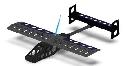
Answer: In the example shown, the wing aero profile extends across the top of the fuselage and is therefore subject to the 0.25 inch clearance rule. If the release mechanism connects to the wing, it must extend a minimum of 0.25 inches away from the fuselage to be compliant.
