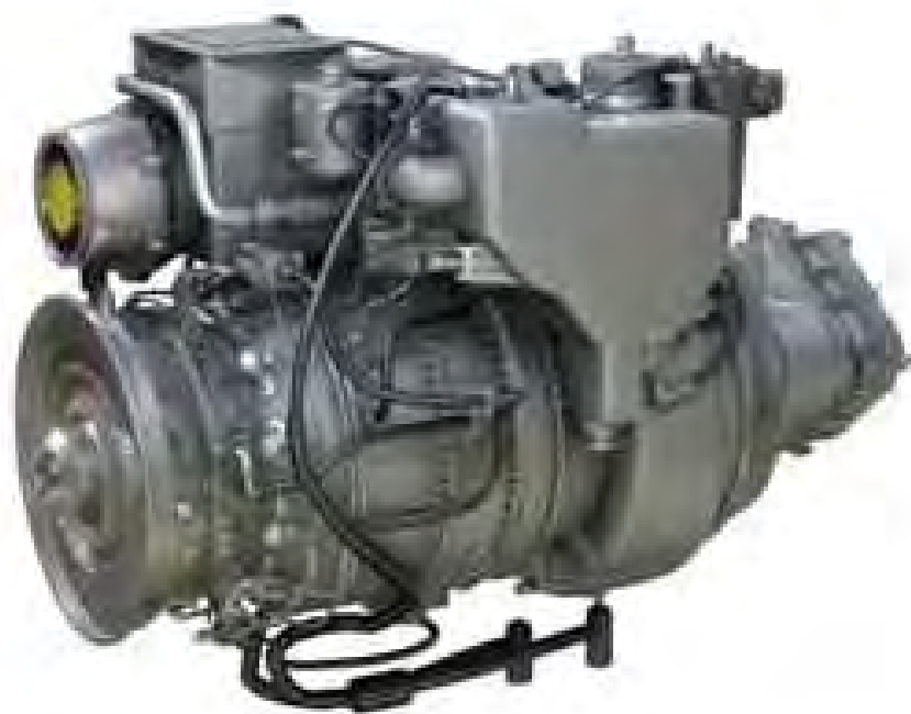
Figure 15: Boundary Layer Control Engine: LHTEC t800
