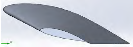
Figure 19: NACA 65 Series Wing at High Angle of Attack
