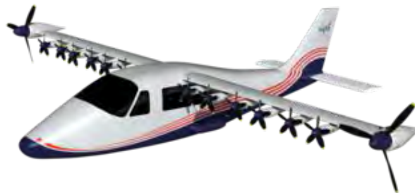
Figure 3: NASA is currently investigating DEP on a test aircraft called the X-57 Maxwell 29
