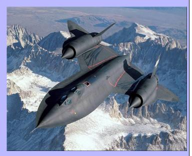
angle; this lowers the drag when the airplane is flying at its cruising speed. Finally, look at the SR-71. Its wings are triangular in shape; this is called a "delta wing" after the Greek letter "delta," which is shaped (as a capital letter) as a triangle. This is the best shape for an airplane which spends most of its time flying faster than the speed of sound.
