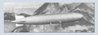
cargo. Because of this, most of the Graf Zeppelin was made up a large bag of this gas—776 feet long and 80 feet in diameter—and only a little bit at the bottom, called the "gondola," was the Graf Zeppelin's cargo. Engines onboard the Graf Zeppelin powered propellers allowing it to move around where its crew wanted it to go. The propellers were mounted in the back of the airship pushing it forward; movable fins in the back allowed it to be steered in whatever direction the pilot directed it.
