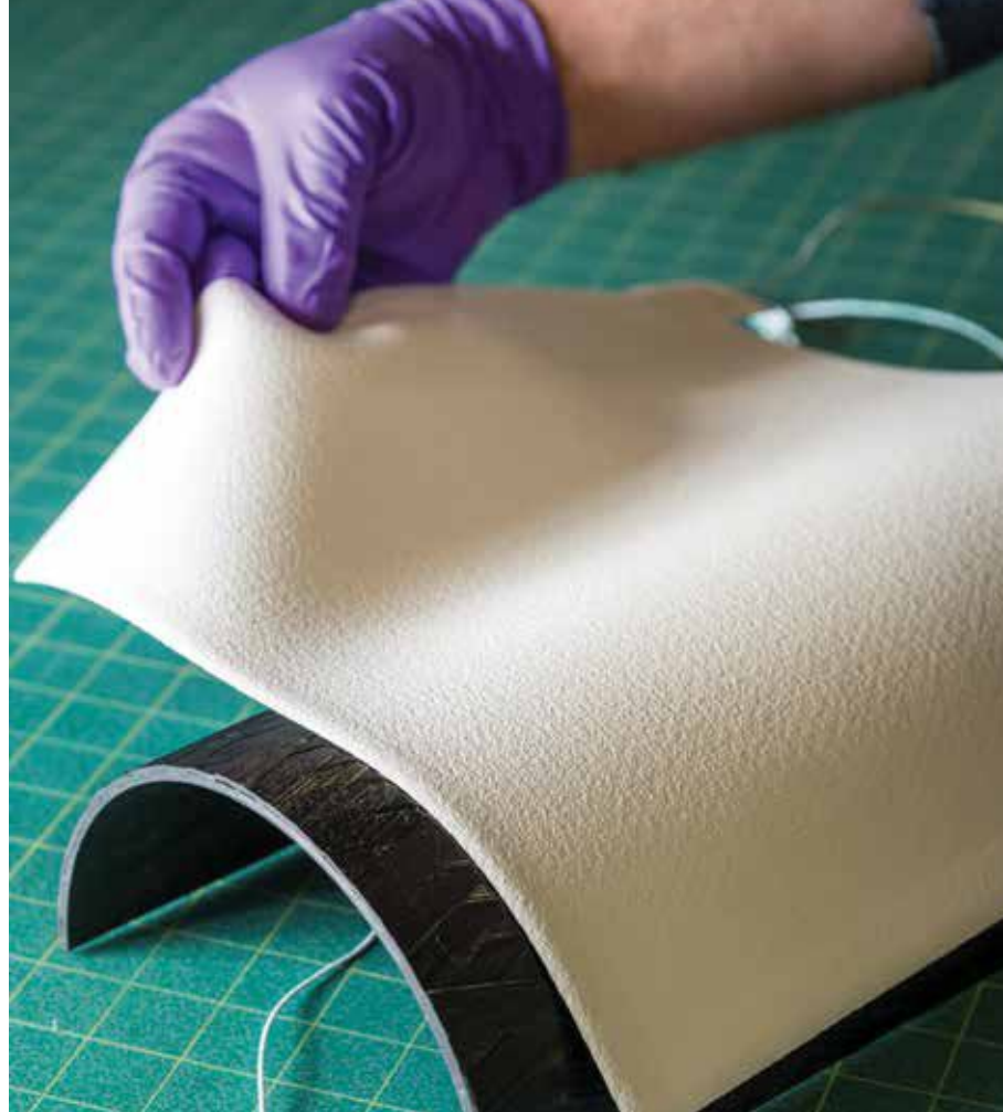
▲ Heating blankets made of nanotubes can aid in the manufacture and repair of composite materials reinforced by carbon fibers. Veelo
