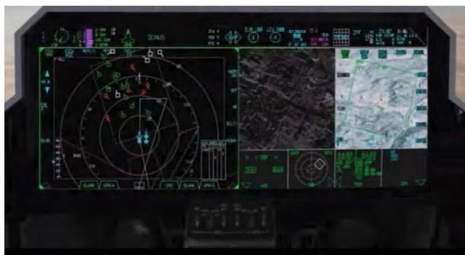
**Figure 12.4:** AN/APG-81 Displays on Glass Cockpit [58]
