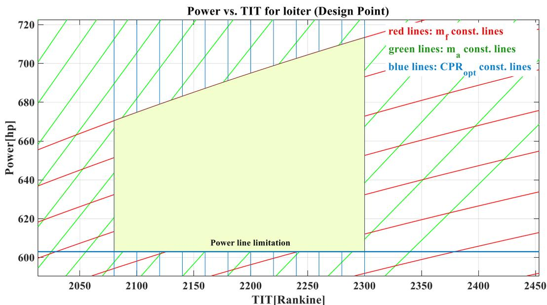
Figure 2.7: Allowable Design Area at Loiter
