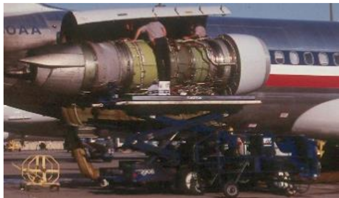
Figure 7-12: Easy Line Maintenance for Engine at 10 ft off Ramp like Skyblazer, DC-9, EMB-145, and CRJ [31]
