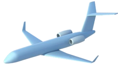
Figure 7-10: Low Wing/Aft Engines
