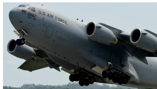
Figure 7-14: C-17 Globemaster II Landing Gear and Fuel Sponsons [32]
