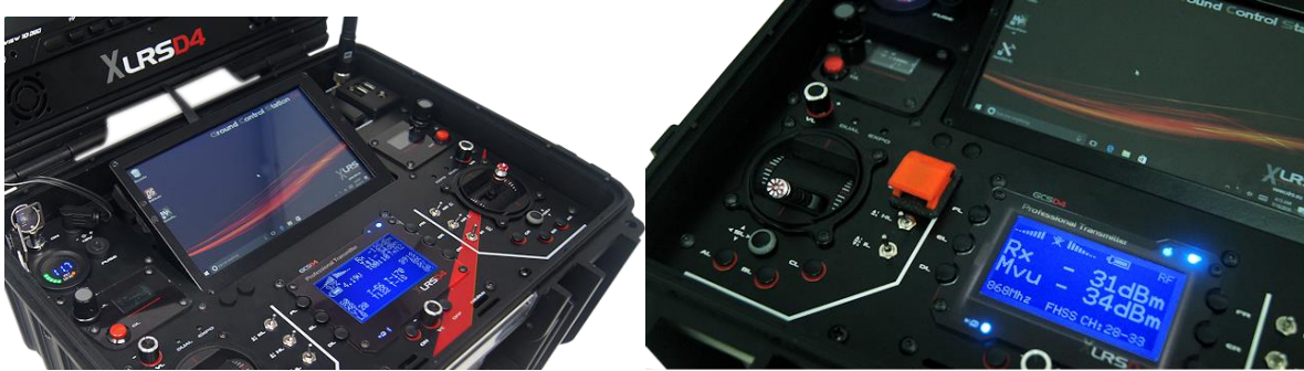
Figure 14-5 GCSD4 | Left: RC control view | Right: Safety control switch
