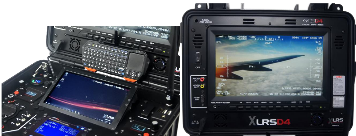
Figure 14-6 GCSD4 | Left: Embedded PC | Right: FPV Video Screen
