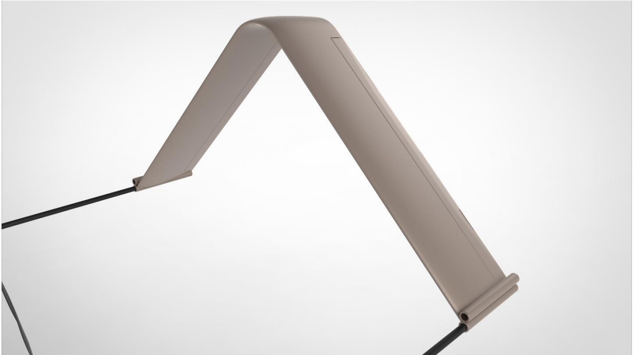
Figure 6–2 WAAPI UAV twin boom inverted V
