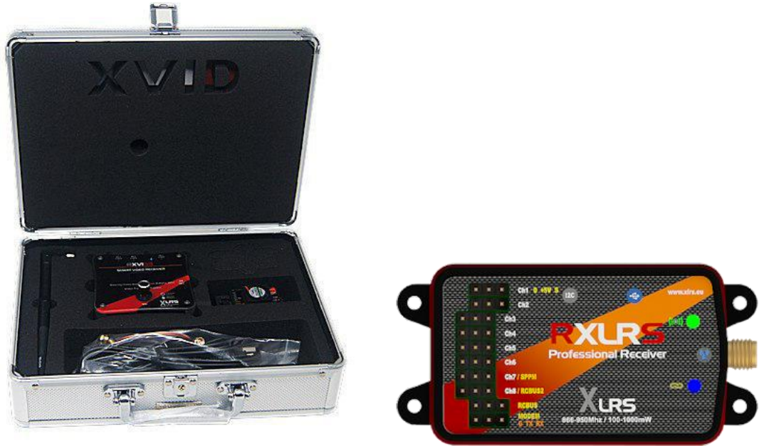
Figure 14-9 GCSD4 | Left: XVID3 Analog Video System | Right: Professional radio control receiver
