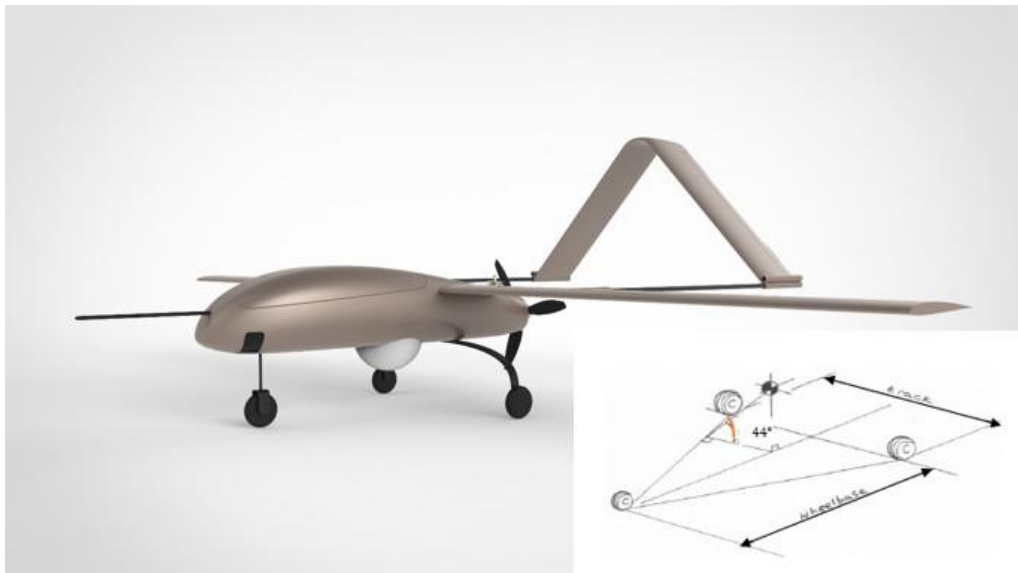
Figure 9–12 Tricycle landing gear geometry
