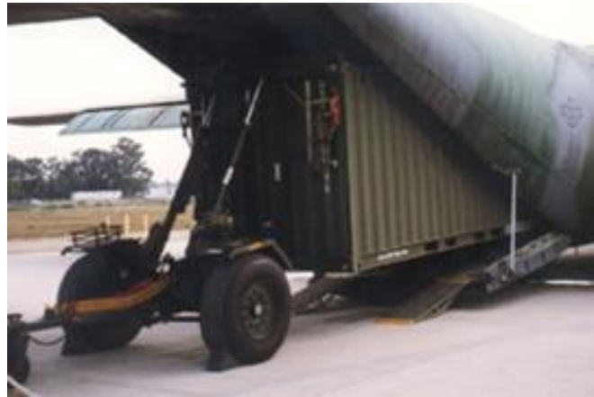
Figure 1.0-1: ISO 20 ft Container loading of a C-130 1
