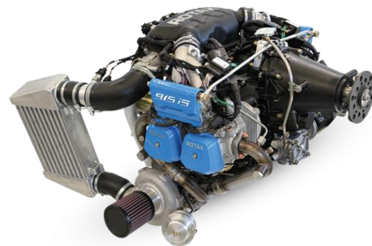
Figure 6.3: Rotax 915iS Engine [31]
