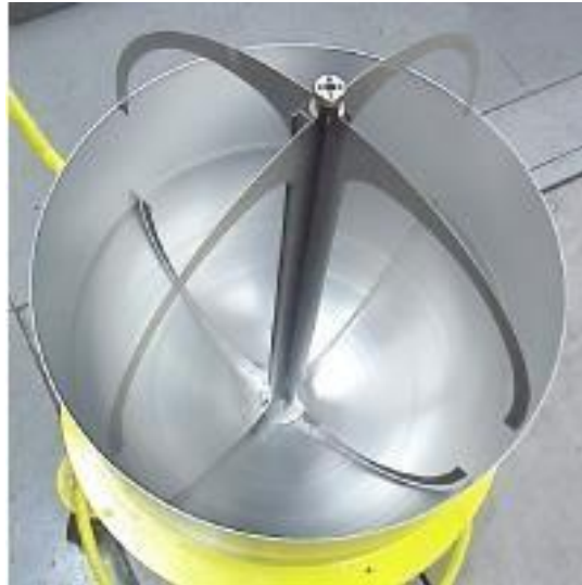
Figure 19. ALMA’s tanks use an all titanium PMD. The PMD uses simple vane technology to allow propellants to flow “uphill” against the acceleration of the spacecraft, ensuring continuous flow of propellant 29 .
