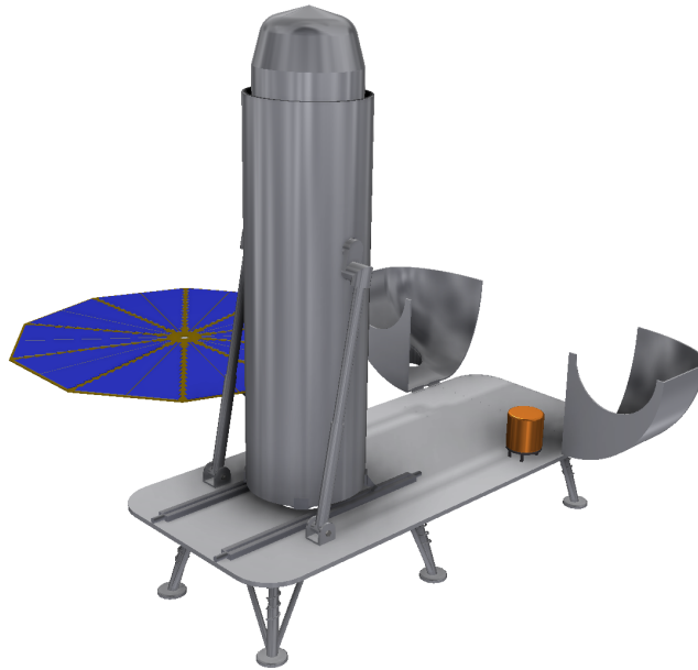
Figure 7.4: MAV is tilt to its vertical launch position with OS in payload bay and nose cone sealed to second stage.
