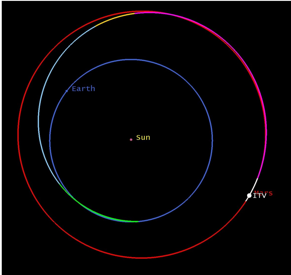
Figure 4.3: A two-dimensional view of the Earth to Mars low-thrust trajectory modeled in STK. Initial conditions are the escape parameters of Earth launch, and the final conditions are when the ITV has achieved a stable, highly elliptical orbit about Mars. The total flight time is 1.4 years with a total delta-V of 3.6 km/s and 345 kg of xenon fuel consumed. The trajectory consists of an initial 60-day coast period followed by 4 main burn segments differentiated by color and detailed in the accompanying table.
