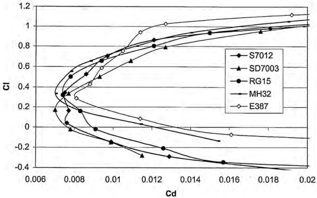
Figure 4.4 Airfoil comparison at  $Re = 300K$
