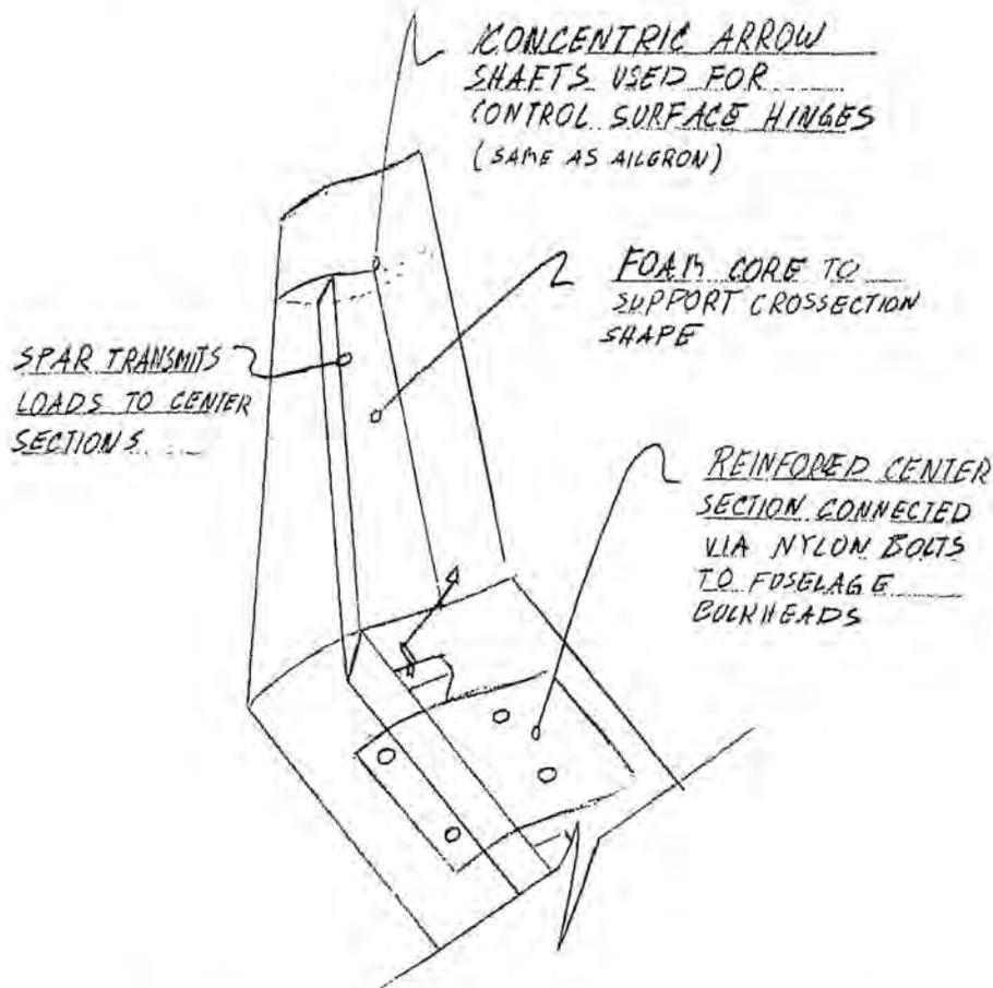
Figure 7: Final Conceptual Sketch of the Tail Structure
