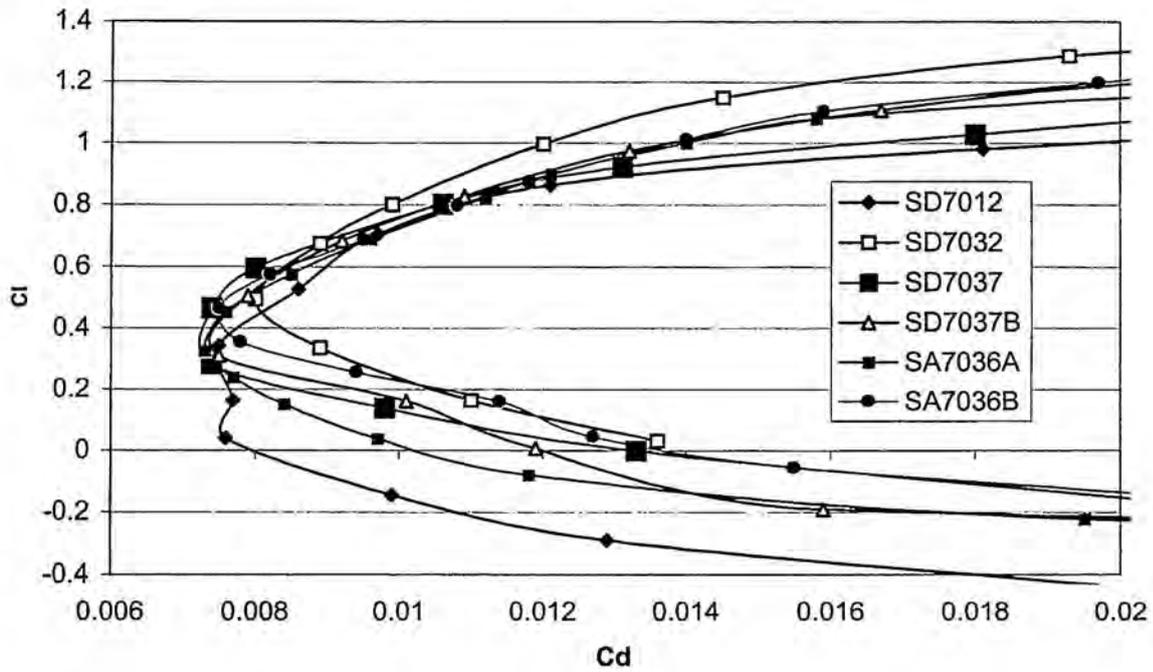
Figure 5.2 Airfoils evaluated for wing tip at Re=300K
