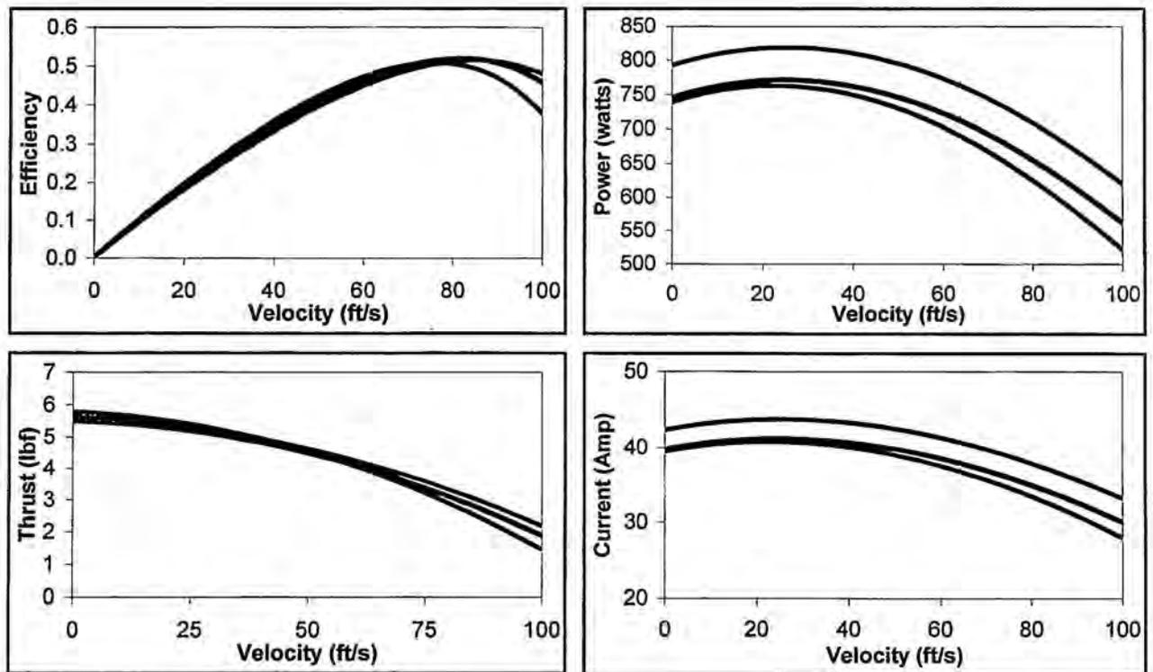
**Figure 13: FAI Motor Performance Data. From top left clockwise: Efficiency, power available from the batteries, current, and takeoff thrust. Blue represents the FAI 25 motor, red represents the FAI 40 p/n 642 motor, and black represents the FAI 40 p/n 643 motor.**
