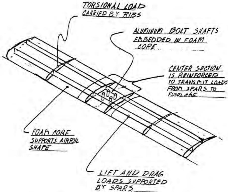
**Figure 6: Final Conceptual Sketch of Wing Structure**
