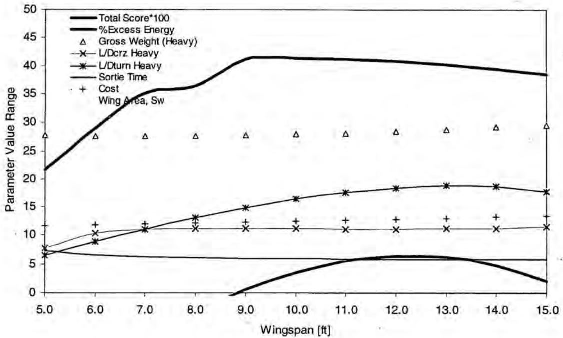
Figure 4.2 Wingspan trade study showing optimum  $b_w = 9$  ft.
