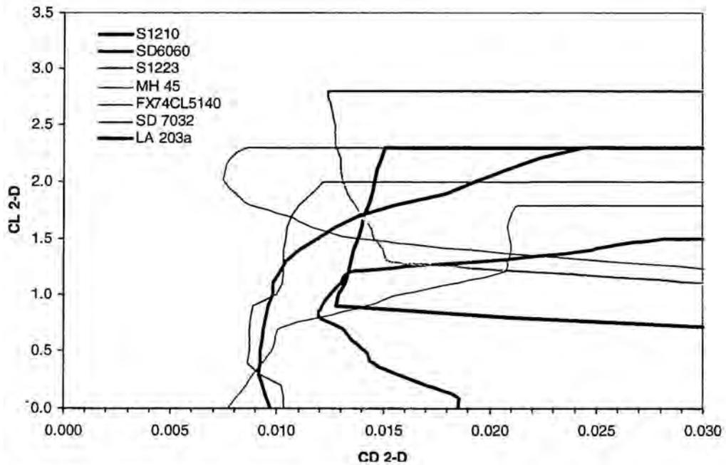
**Figure 4.1 Airfoil drag polars, including geared flap effects.**
