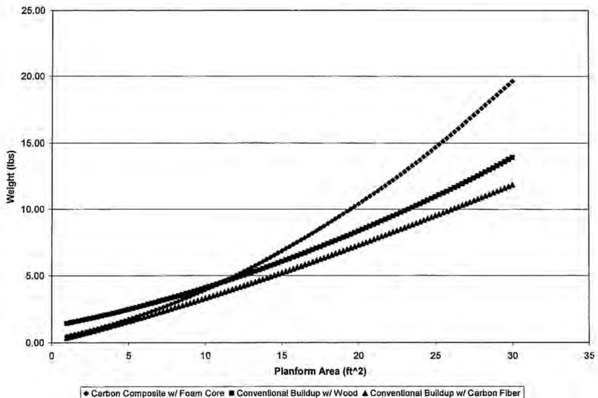
**Figure 5: Wing and Tail Structural Material Comparison**
