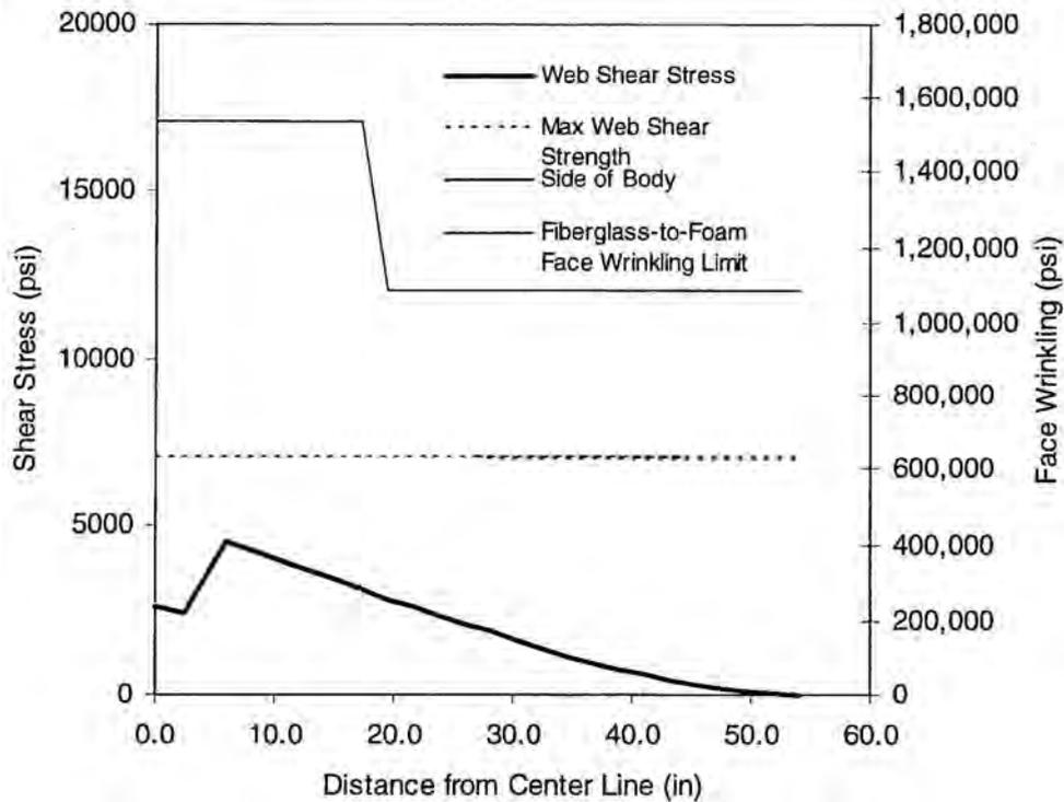
Figure 4.9. D-section shear and face wrinkling behavior.
