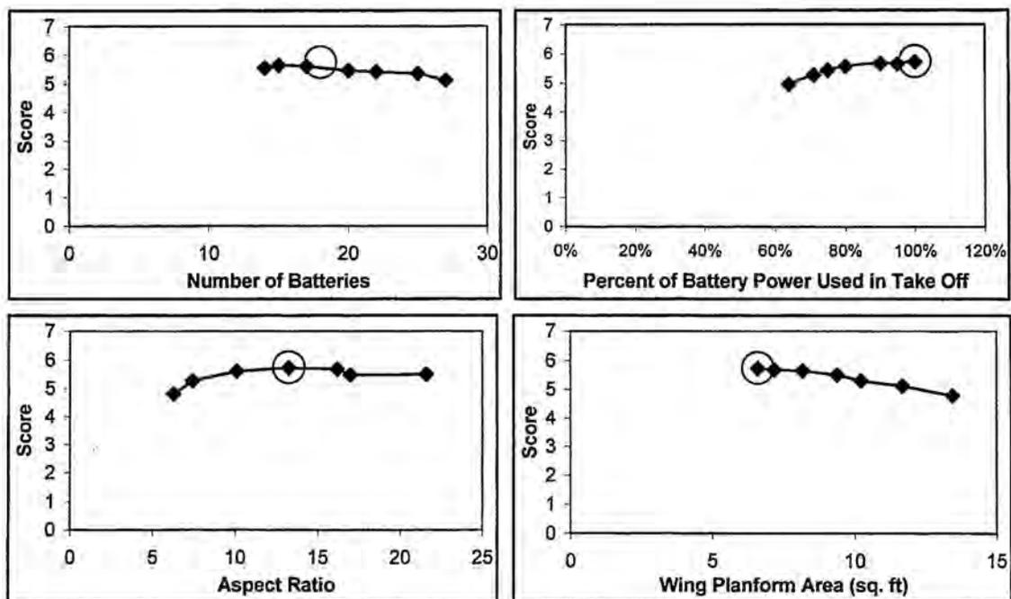
**Figure 10: Tradeoff Analysis Results. From top left clockwise: Number of batteries required, takeoff power required as a percent of available power, wing planform area requirement, and aspect ratio requirement. Red circle represents the optimal value found by the program.**
