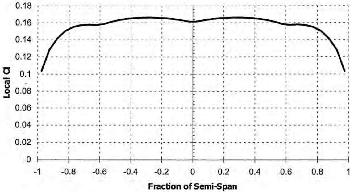
Figure 5.1 Span wise Cl distribution for final wing planform
