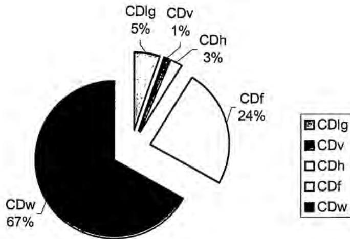
Figure 4.7 Drag breakdown at end of 3<sup>rd</sup> 180 deg for passenger delivery
