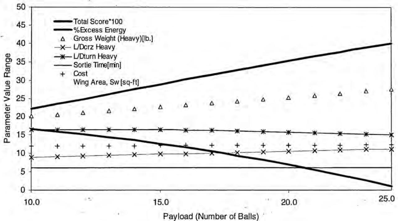
Figure 3.3. Payload capacity trade study results.
