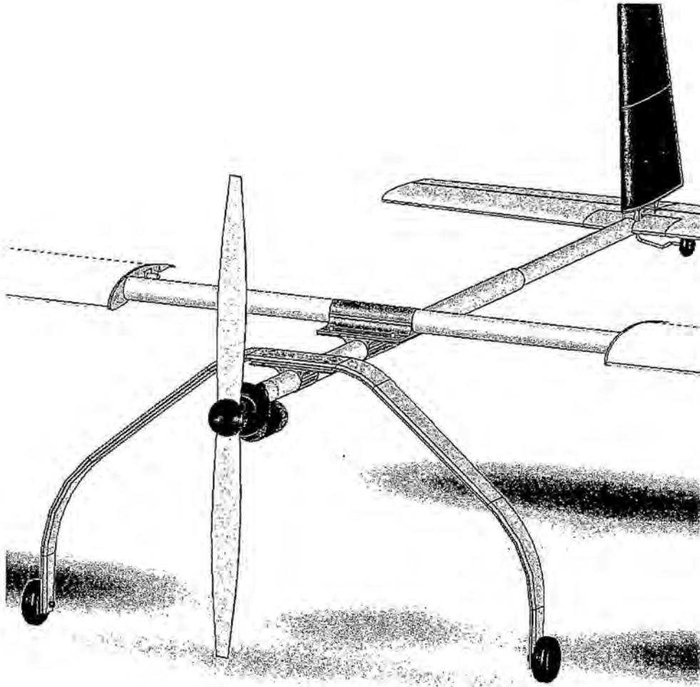
**Figure 4.2.15 Joint connecting wing spar and landing gear to backbone**
