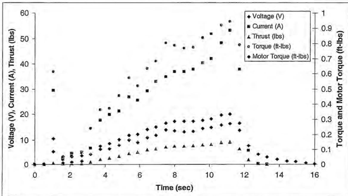
Figure 7.1.2 Time trace for CP 1300's with a 22x14 prop and 3.5 gear ratio.
