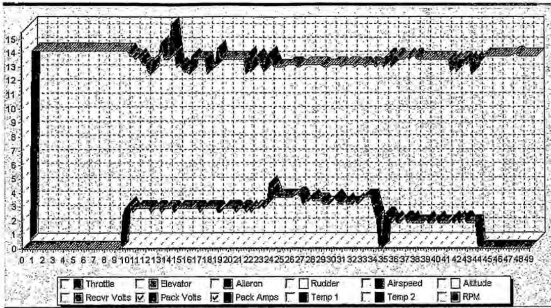
Figure 7.1.7 Flight Data Recorder graph showing voltage and current.
