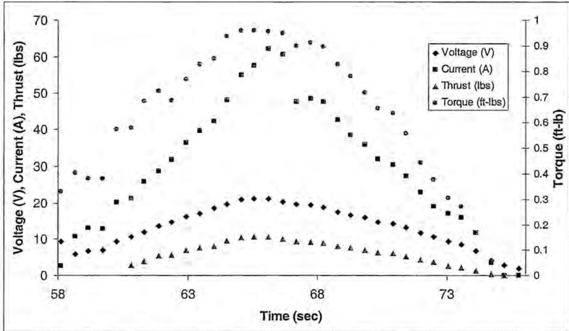
Figure 7.1.1 Time trace of the data for the Graupner 930-10 with the competition prop (zinger 22x14)
