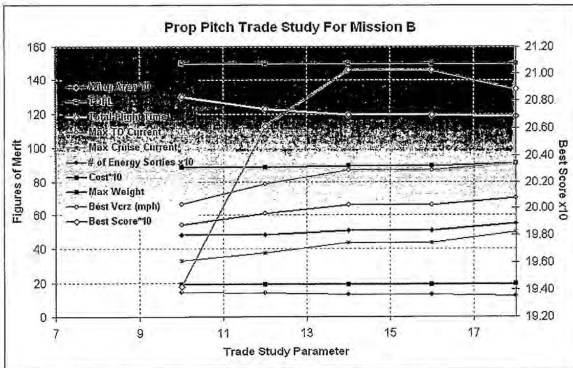
Figure 4.2.8 Trade Study of several Figures of Merit vs. prop pitch. Trade Study Parameter is prop pitch in inches
