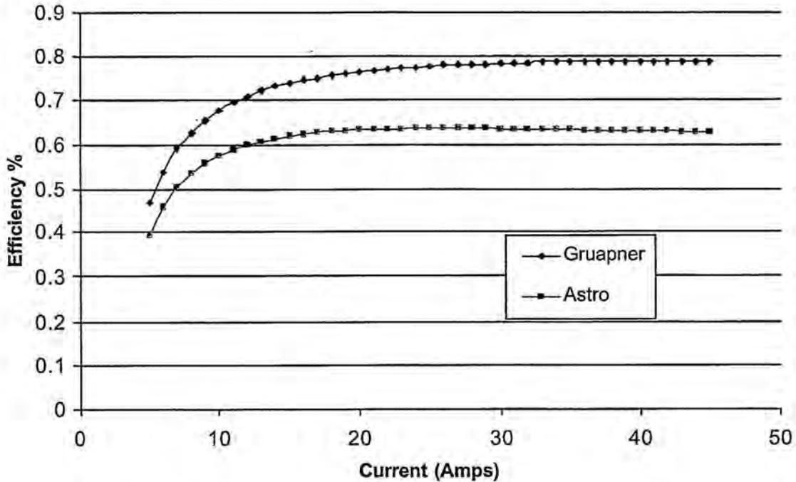
Figure 4.4: Efficiency versus Current for Graupner
