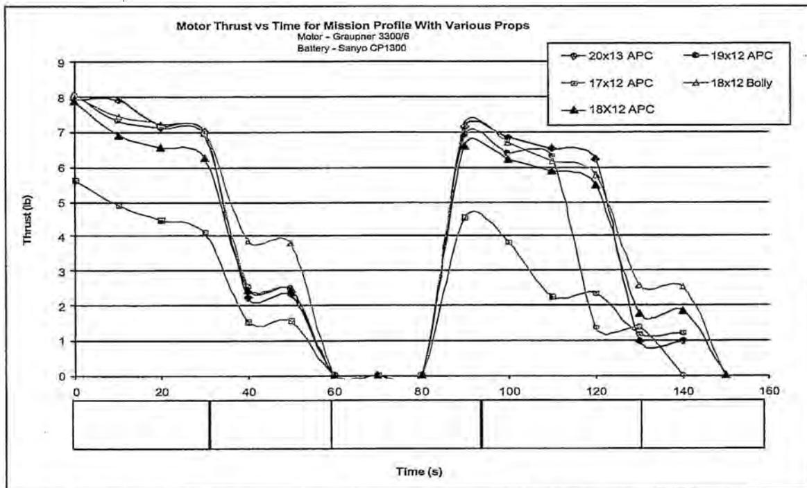
Figure 4.11: Mission Profile Using Optimized Propeller and Gearbox Configurations
