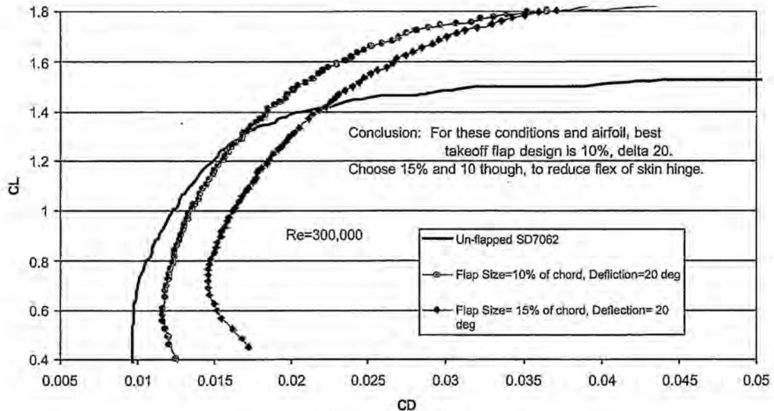
Figure 4.5: Flap Size Determination
