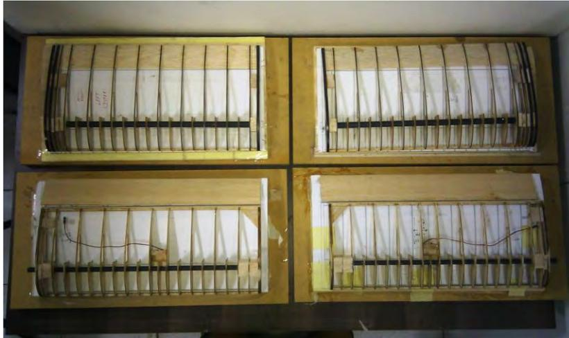
Figure 20: Four sections of the main wing in construction.
