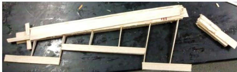
Figure 8.4: Broken full wing with D-tube.
