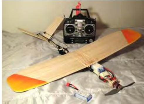
Figure 37: Test bed airplane used for airborne battery testing.
