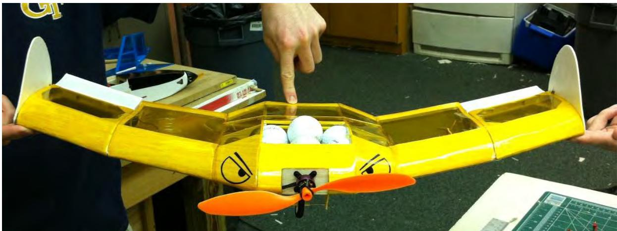
Figure 8.3: Wingtip structural test with full payload
