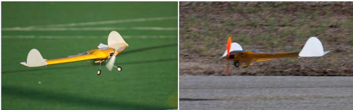
**Figure 4.13:** Comparison of prototype aircraft with different styles of landing gear
