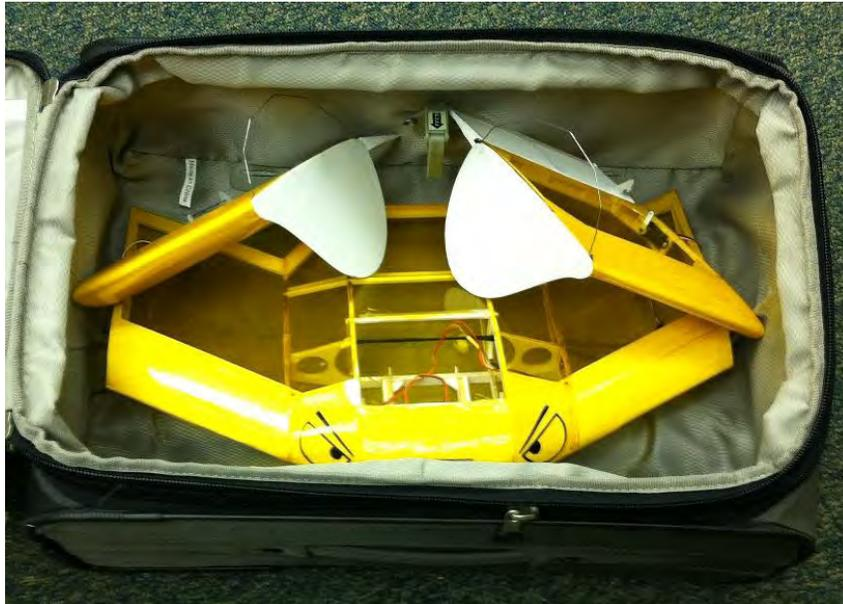
**Figure 5.4:** The aircraft unassembled to fit in the suitcase
