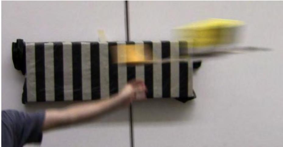
**Figure 4.1:** Testing hand-launch velocities
