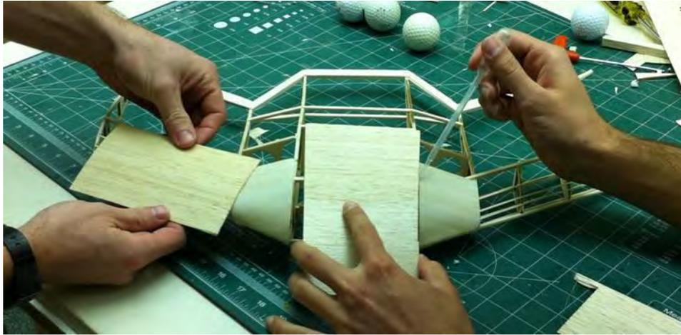
**Figure 6.1:** The team fitting balsa sheeting to the aircraft
