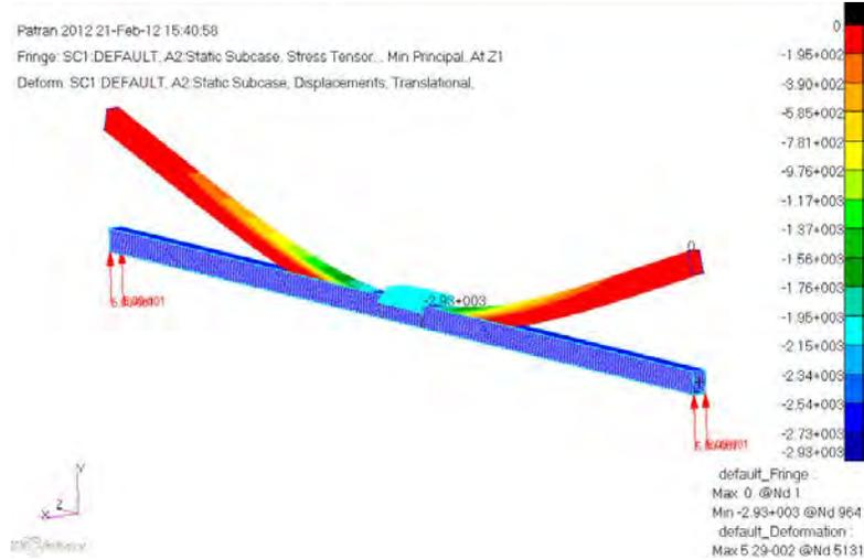
**Figure 5.8: Compressive stress (psi) on the wing spar due to a 5 G load**
