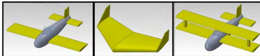
**Figure 3.4: Aircraft Configurations**
