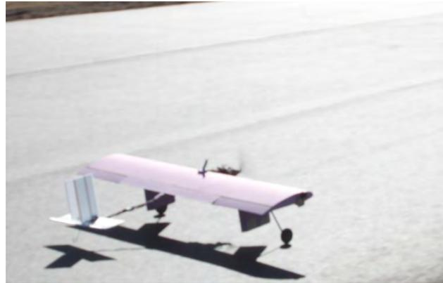
**b) Initial Foam Prototype During Takeoff**
