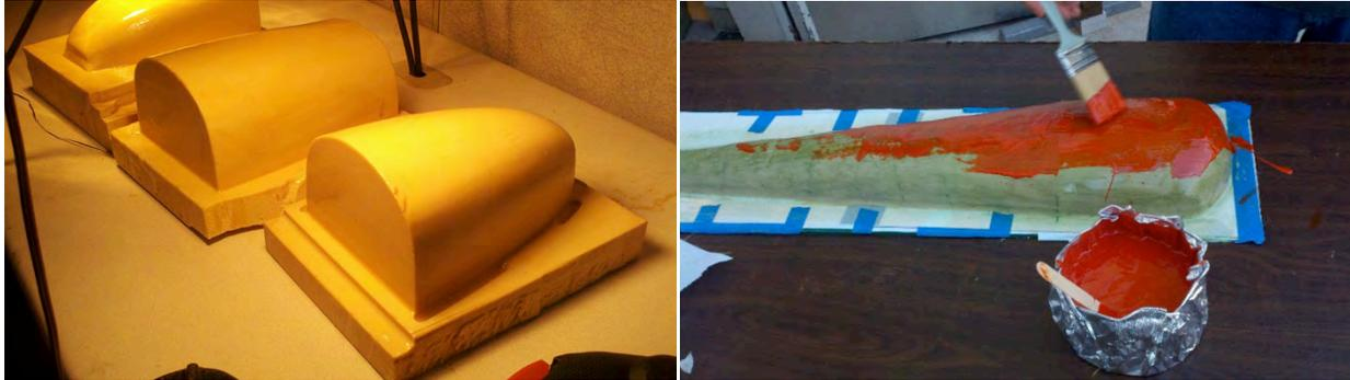
**Figure 6.2: CNC cut fuselage molds (Left), tooling gel mold making (Right)**
