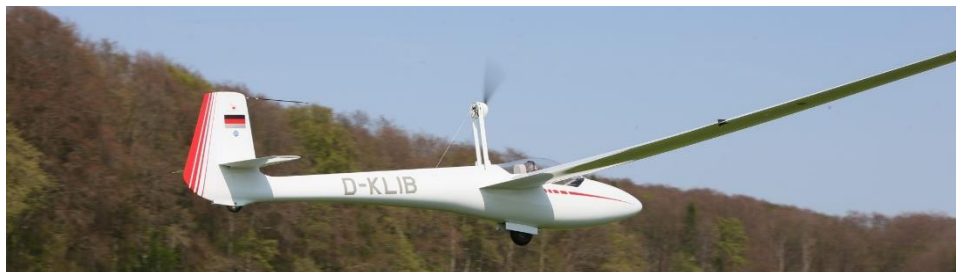
Glasflugel elibelle, a self-launching glider equipped with a retractable electric propulsion system. ( https://streiflyshop.de/wp-content/uploads/2023/03/CPF24214-1920x1280.jpg )
