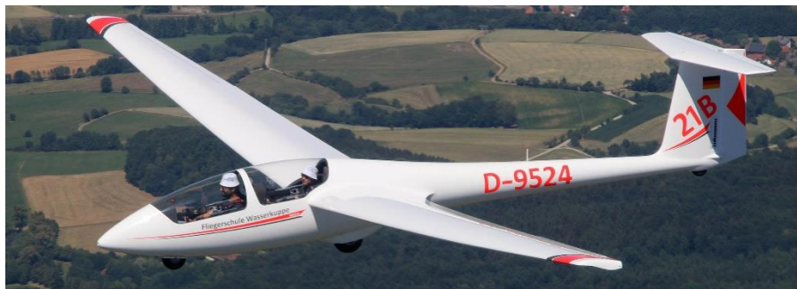
Schleicher ASK-21, a modern composite training glider. ( https://www.alexander-schleicher.de/wp-content/uploads/2018/07/21B-001-Luftbild-010.jpg )
