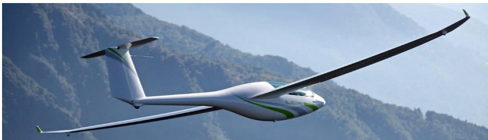
Alisport Silent Electro, a single seat self-launching glider with a folding nose mounted propeller (https://static.homepagetool.ch/var/m_7/75/75e/253592/11444417-DIA_home3-c9f0f.jpg)
