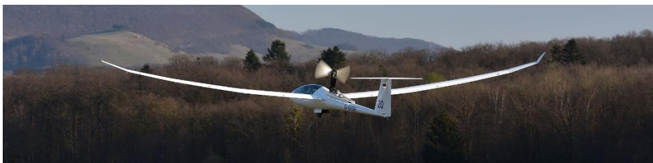
Schempp-Hirth Arcus M, a two seat self-launching racing sailplane, equipped with a retractable two cycle engine. (https://www.schempp-hirth.com/fileadmin/_processed_/a/4/csm_b1948-RS6577_DSC_2264_f9d50bc81e.jpg)
