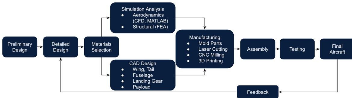
Figure 5: Overall Manufacturing Flowchart
