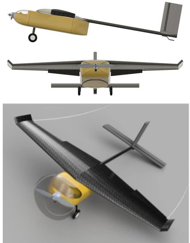
Figure 4: Preliminary model of aircraft
