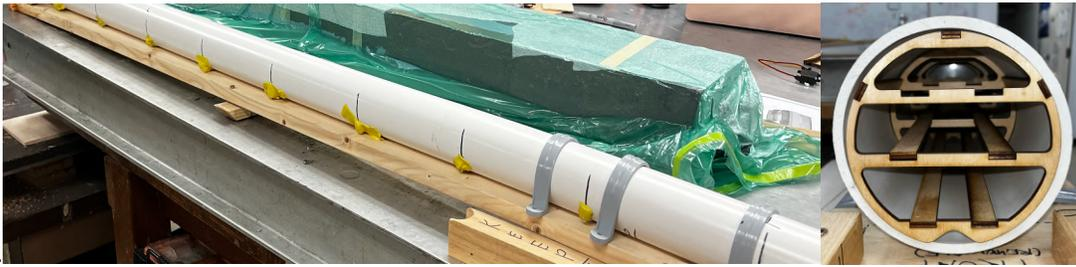
**Figure 44.** 7.00 ft (2.13 m) steamer for longerons (left), internals of 2.00 x 0.5 ft (0.61 x 0.15 m) steamer for balsa sheeting (right)
