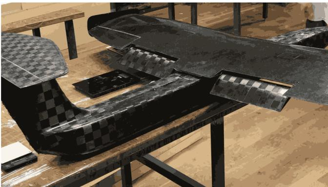
Figure 45: Extended Fowler flaps in the main wing
