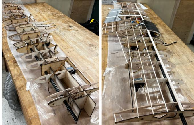
**Figure 45.** Ribs in jig adhered to spar (left), and wing structure after stringer attachment (right)
