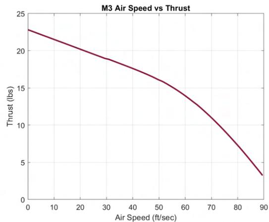
(b) M3 Airspeed vs Thrust
