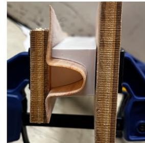
**Figure 47.** Steamed balsa sheet formed in mold
