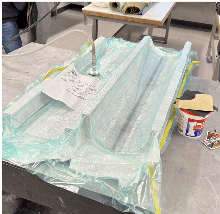
Figure 35: Carbon Fiber Fuselage Layup in Vacuum Bag
