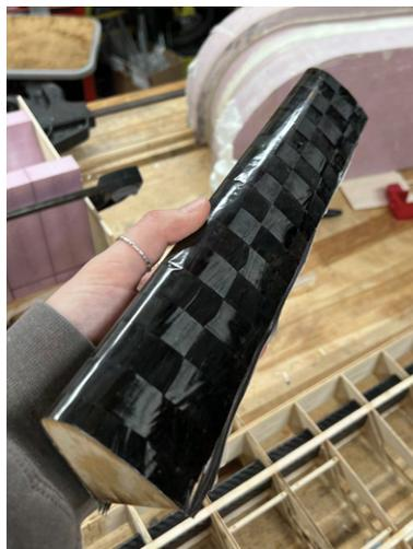
Figure 33: Carbon Fiber, Foam-Core Leading Edge
