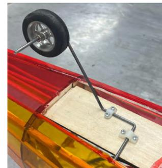
**Figure 51.** Nose gear integration
