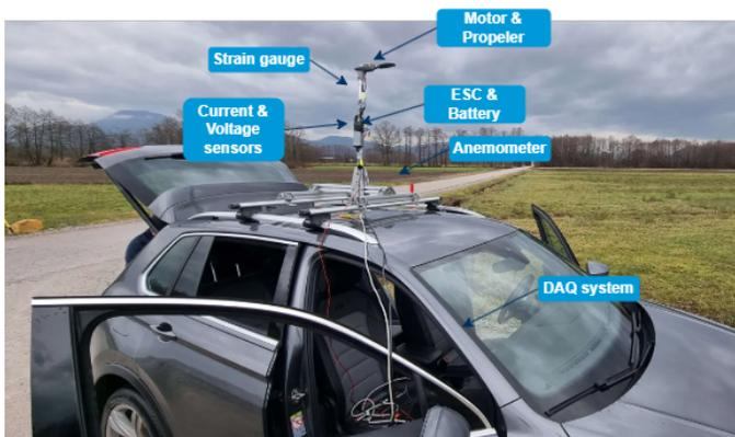
Figure 49: Propulsion testing rig
