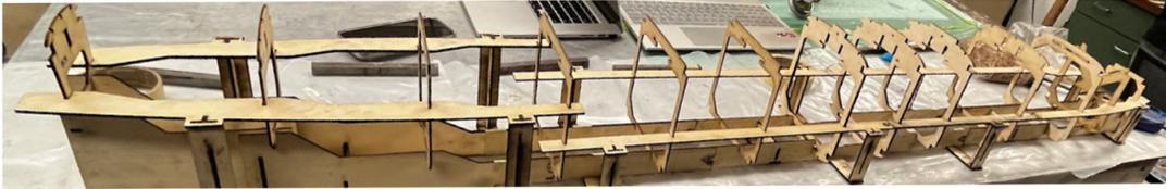
**Figure 48.** Fuselage jig with formers before longeron attachment
