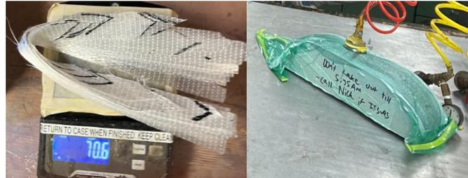
**Figure 49.** Bow gear manufacturing with fiberglass weight (left) and vacuum-bagged layup (right)
