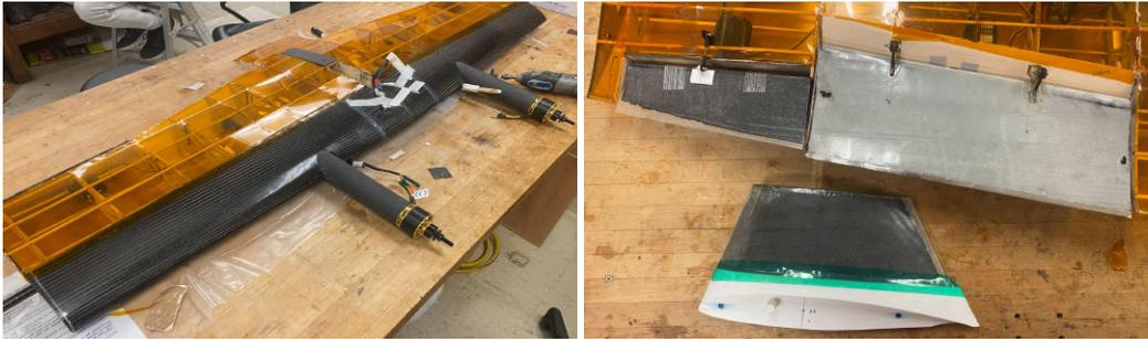
**Figure 46.** Solite, CFRP skin, and motor mounts adhered to wing (left), FG reinforced foam flaps, ailerons, winglets (right)
