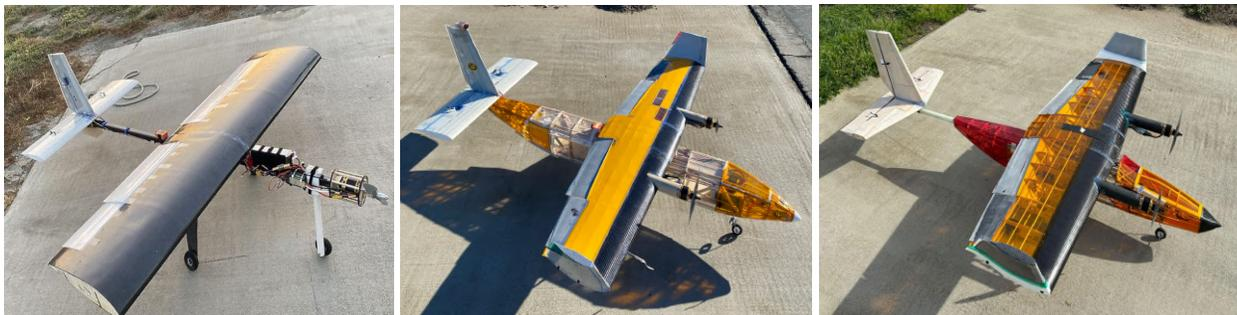
**Figure 67.** From left to right: isometric photos of V0, V1, and V2 at various flight tests.
