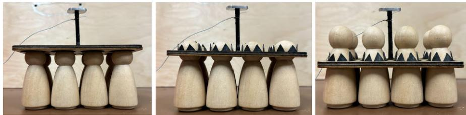
**Figure 40.** Three stages of M3 with 8-Passenger insert loading with inserts placed above Passengers (left), inserts pushed down to open rubber gasket (middle), and Passengers ready for loading (right)
