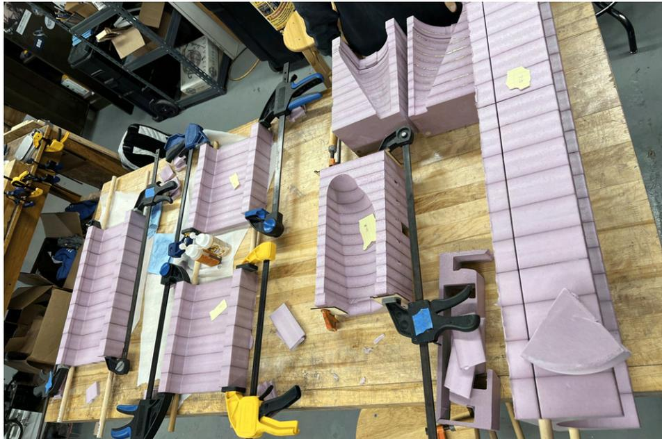
Figure 32: Bonding Fuselage Molds
