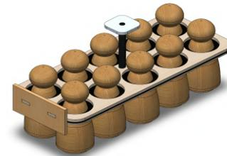
**Figure 39.** Fully loaded 10-Passenger insert with bumper CAD for M3
