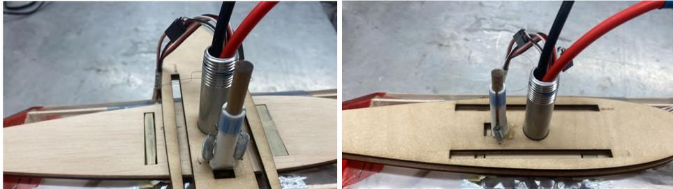
**Figure 32.** Pylon in parking configuration (left) and flight configuration (right)
