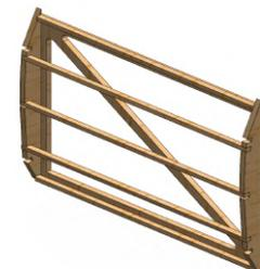
**Figure 41.** Payload hatch (fabric snaps not shown)
