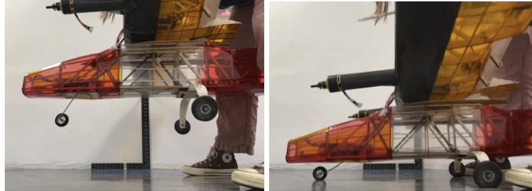
**Figure 62.** V2 fuselage drop testing from height of 8 in (20.3 cm)
