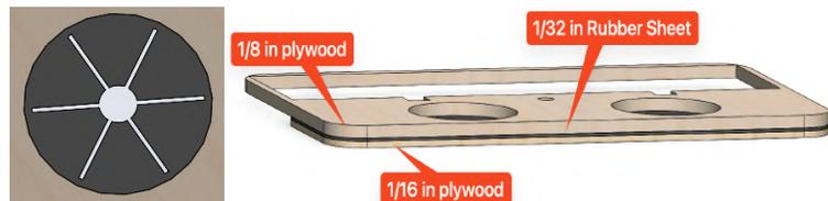
**Figure 52.** Top-down view of a cutout for EMTs or Passengers (left), and M2 Patient + EMT sandwich structure insert (right)
