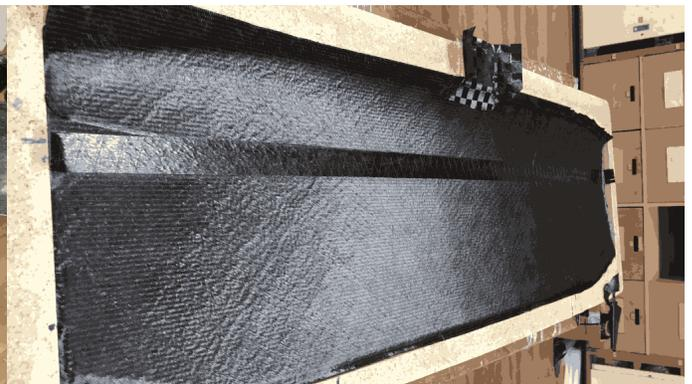
Figure 46: Main wing lamination
