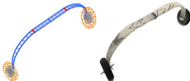
**Figure 33.** GearSizer model of the landing gear (left) and constructed fiberglass gear (right)
