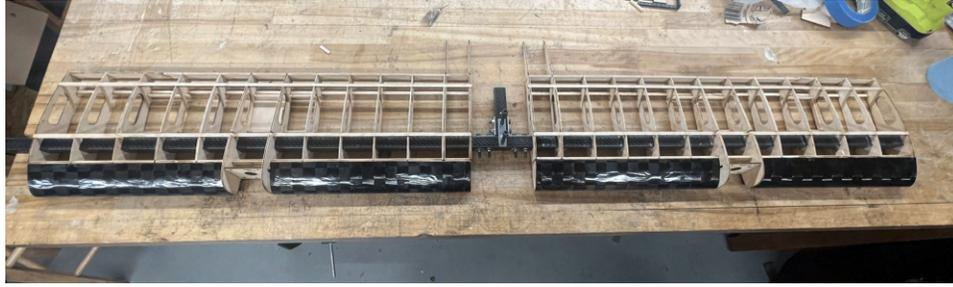
Figure 34: Main Wing Assembly
