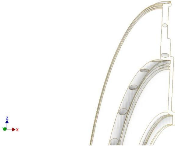
Fig. 4.7. Model 3D of compressor diffuser
