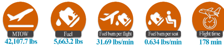
Figure 19- Main output data of the 1000 nmi economic mission performed by the Chaka-50
