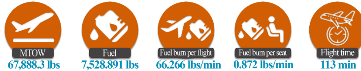
Figure 20- Main output data of the 500 nmi economic mission performed by the Chaka-76
