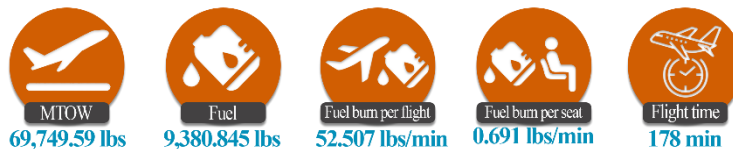
Figure 21- Main output data of the 1000 nmi economic mission performed by the Chaka-76
