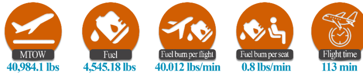
Figure 18- Main output data of the 500 nmi economic mission performed by the Chaka-50
