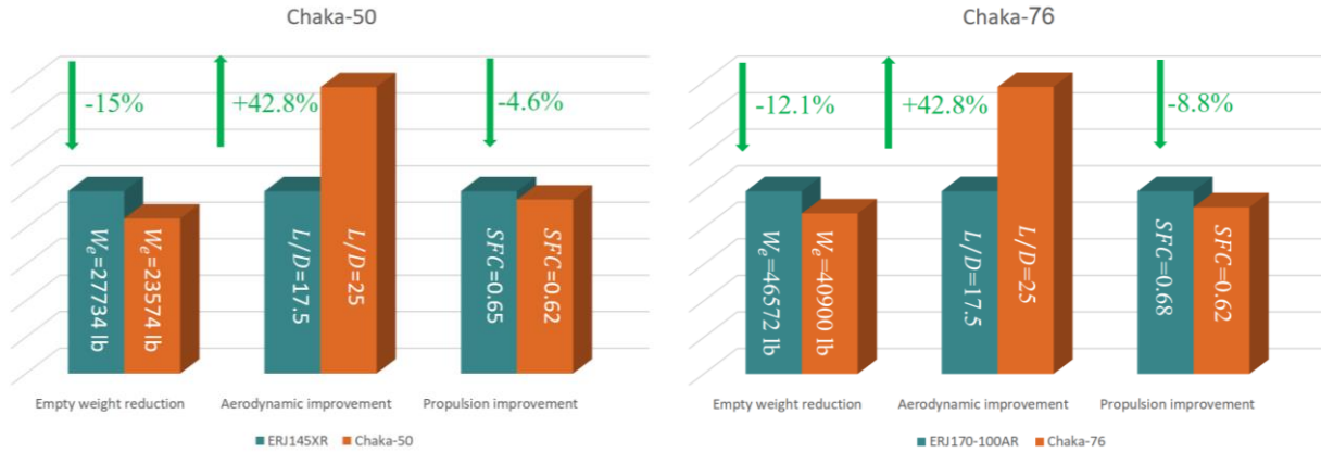
Figure 22- Amelioration occurred in terms of the three disciplines for the Chaka MRJ family compared with competitive RJs
