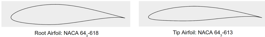
Figure VII-1. Airfoil Profiles of Root NACA 64 3 -618 and Tip NACA 64 3 -613
