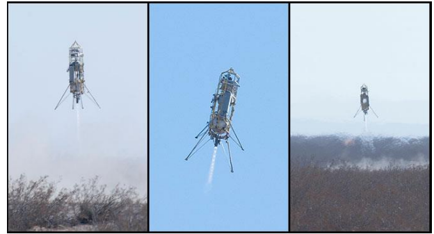
Masten Space Systems' Xombie technology demonstrator lifts off during a flight test of JPL's G-FOLD precision flight control algorithm, autonomously diverts to an alternate landing site, and descends for landing at the alternate site. Credits: NASA / Tom Tschida
