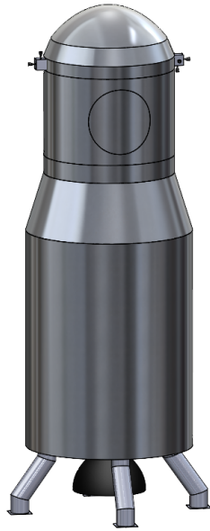
Fig. 20 MAV with hold-down arms and explosive bolts.
