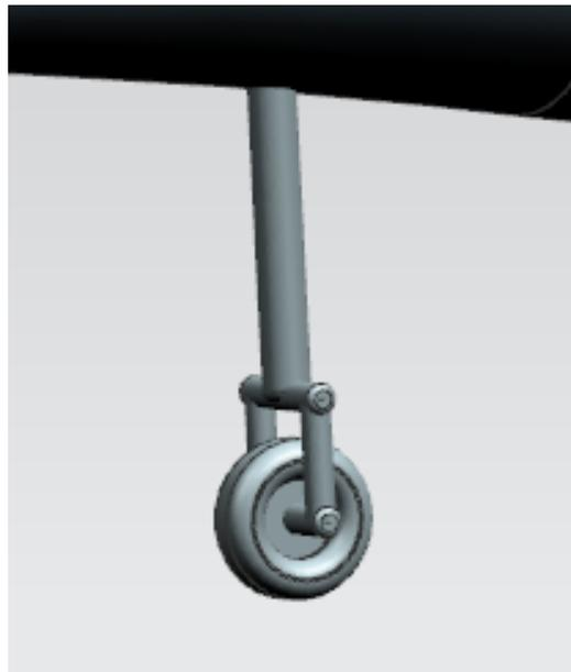
**Figure IX.11:** Nose landing gear of SEAL
