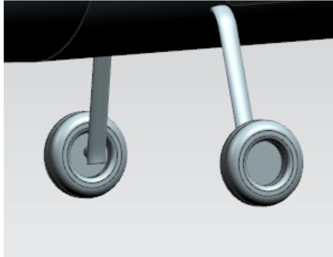
**Figure IX.12:** Main landing gear of SEAL
