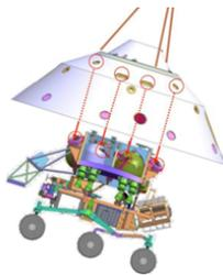
FIGURE 4.7: Original sky crane and back-shell interface.
