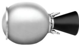
FIGURE 5.6: STAR 13B. First Stage Solid Rocket Motor.
