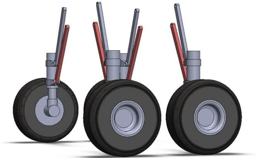
**Figure 12-2 Main Landing Gear**
