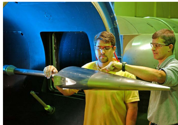
Hypersonic Waverider and Scramjet concepts; aerodynamic validation and verification testing
