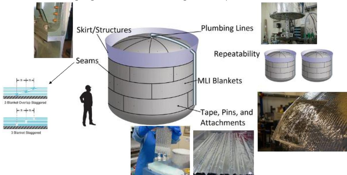
**Fig 1. IFUSI performed thermal characterization testing on MLI systems, epoxies for cryogenic tanks, and assessed thermal repeatability of MLI systems.**
