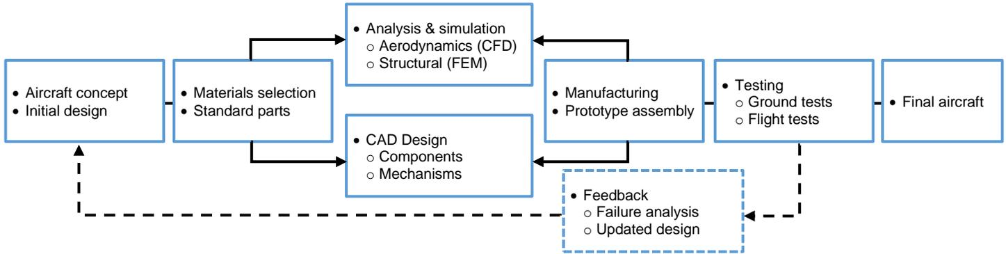
Figure 6: Manufacturing flowchart
