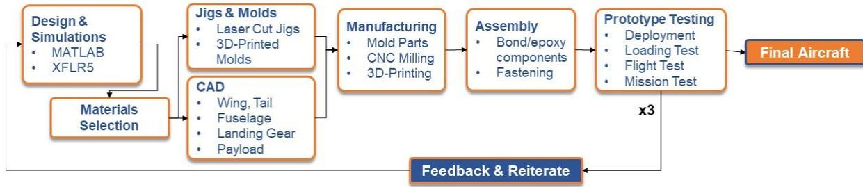
Figure 4.1 – Manufacturing Plan
