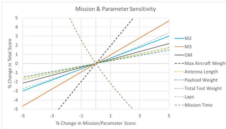
Figure 3.1 – Overall Mission & Parameter Sensitivity
