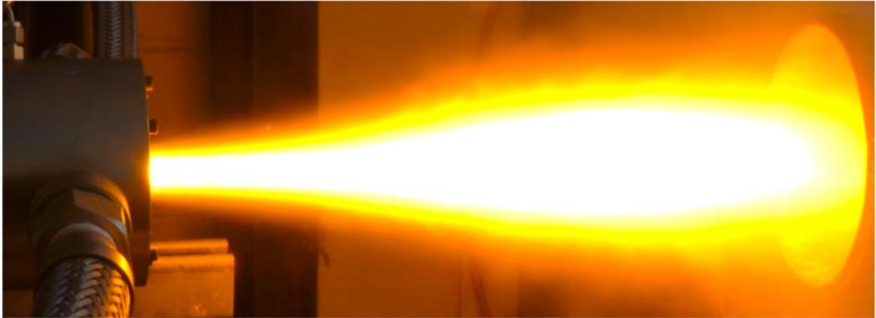
**Figure 22 Purdue University 2-inch Hypergolic Ignition Test**
