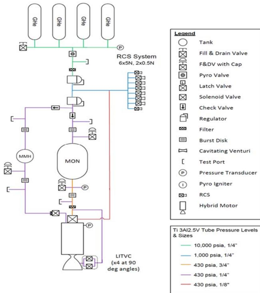
**Figure 24 PAA MAV Hybrid Propulsion System Schematic**
