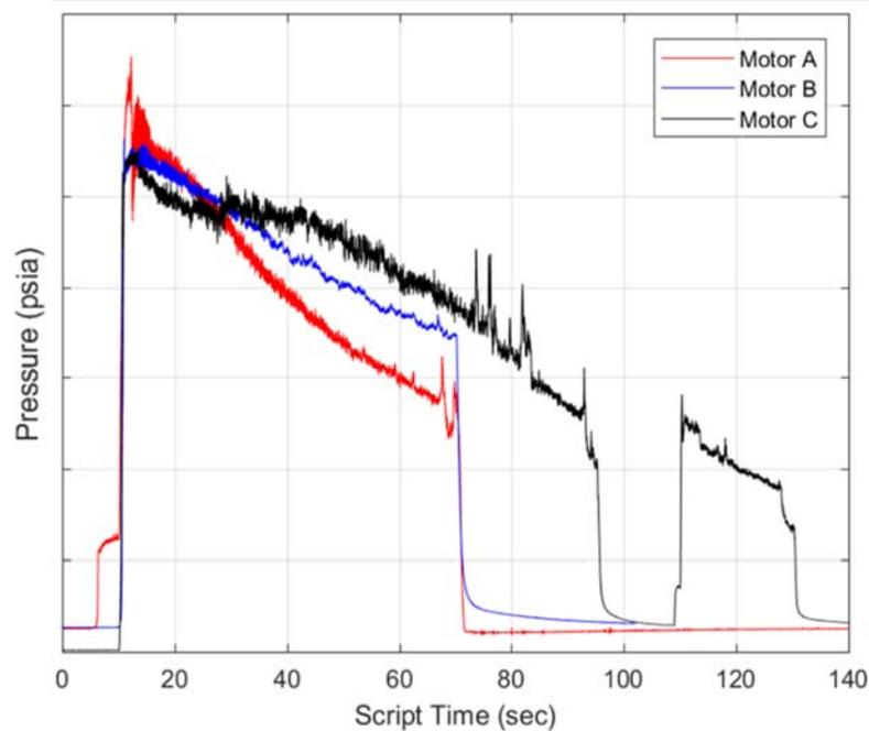
**Figure 18 Whittinghill Aerospace Motor C Chamber Pressure [22]**
