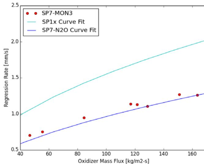
Figure 2 Comparison of Regression Rate Data for SP7/MON-3 With the Curve Fits for SP7/ $N_2O$  and SP1x/ $N_2O$  [10]
