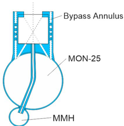
**Figure 15 Cross section view of a hypergolic MON-25/MMH igniter concept.[21]**
