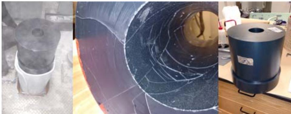
**Figure 9 Processing in the -40C Freezer(left), cracks from warm insulator assembly(middle) and replacement segment (right) for Whittinghill Motor B (FT04)**
