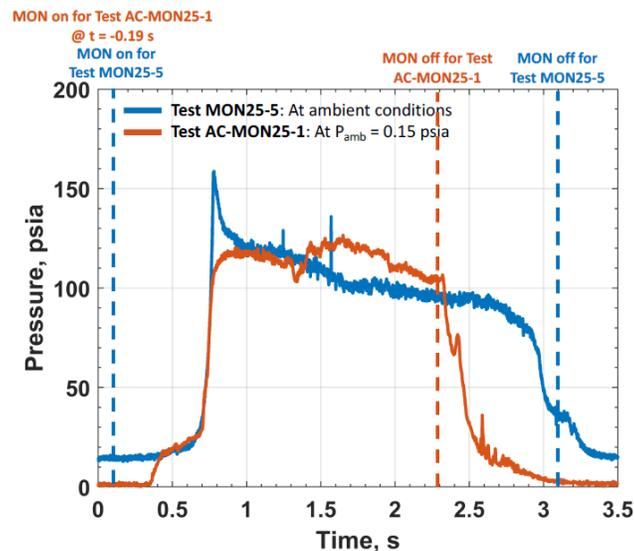
**Figure 23 Purdue University Ground and Altitude Chamber (AC) Start Hypergolic Ignition Tests.**
