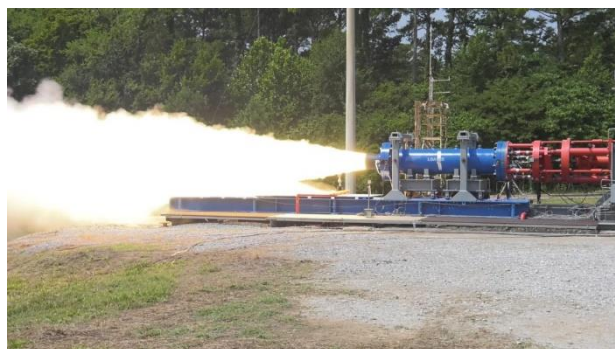
Figure 11. The SLS Program and boosters prime contractor Northrop Grumman have performed subscale motor testing for the Block 2 evolved boosters.
