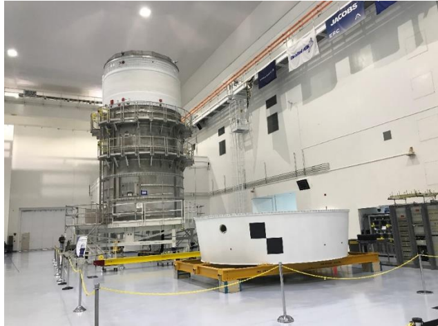
Figure 6. The Artemis I Interim Cryogenic Propulsion Stage (ICPS) and Orion Stage Adapter (OSA) at KSC.
