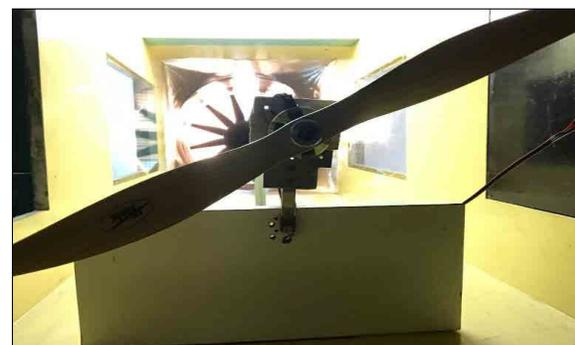
Figure 7.4: Dynamic Thrust Test
