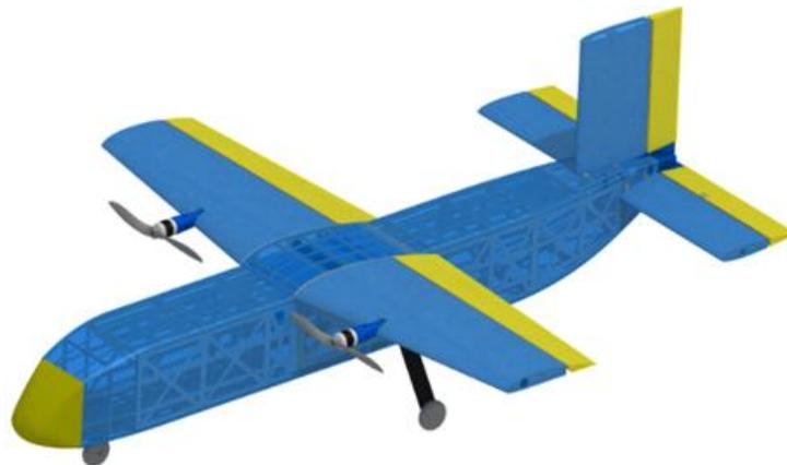
Figure 5-1: Finalized design of the aircraft.
