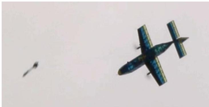
Figure 8-8: Aircraft completing a 360-degree turn with sensor deployed.
