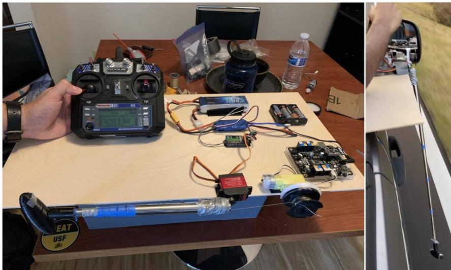
**Figure 7.3: Functional mechanism prototype setup (left) and initial testing out of a car window (right)**
