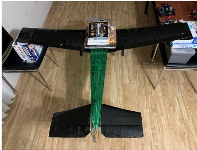
**Figure 8.1: Simulated extreme case wingtip load test**
