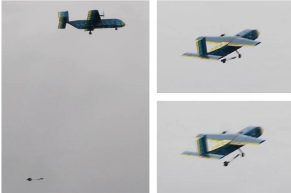
Figure 8-4: Sensor in flight at different tow lengths: 200 in (left) and 6 in (right).
