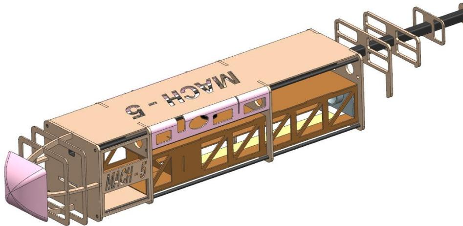
**Figure 25:** Wood Fuselage with Carbon Supports
