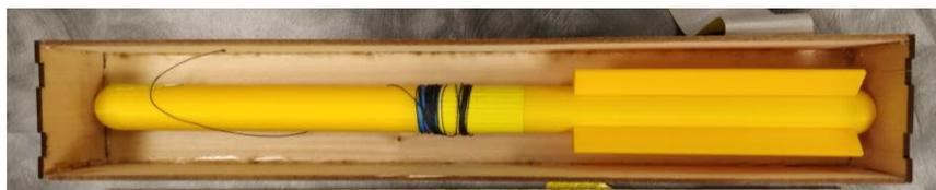
**Figure 43:** Sensor in Container for Drop Testing
