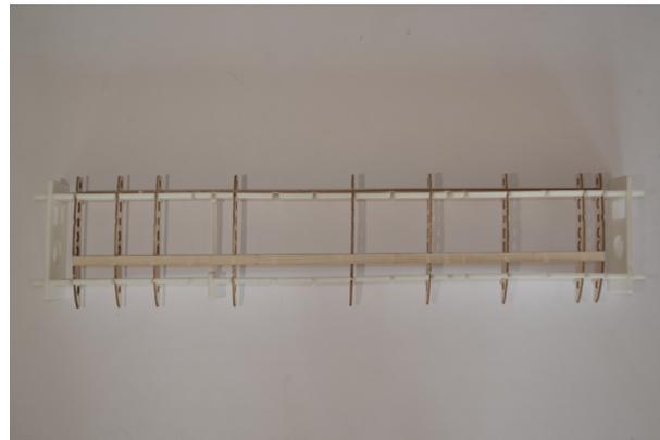
Figure 6.1: Wing construction
