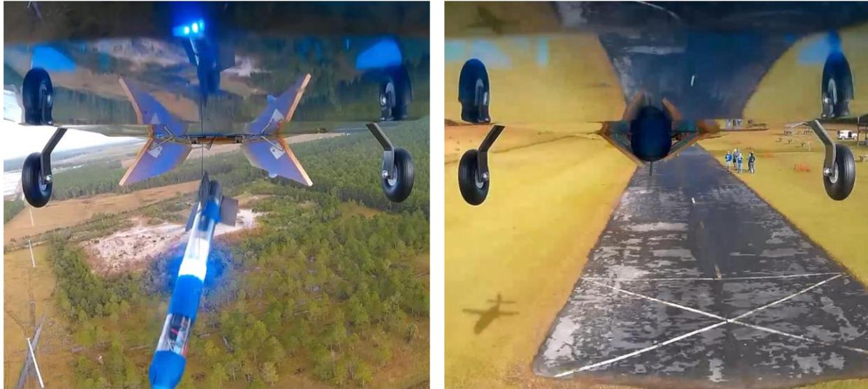
*Figure 8-5: Sensor and bomb bay prototypes during deployment (left) and retraction (right), with blue sensor light visible (left).*
