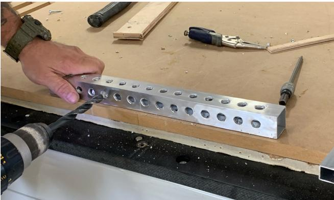
(a) Telescoping rods drilling process
