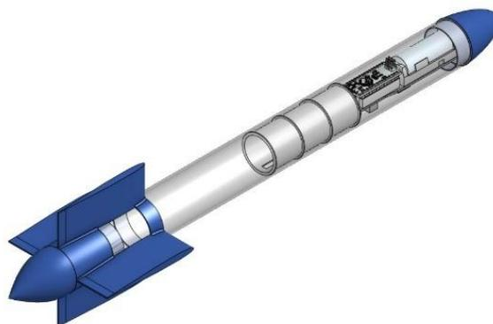
*Figure 5-13: Clear polycarbonate sensor body.*
