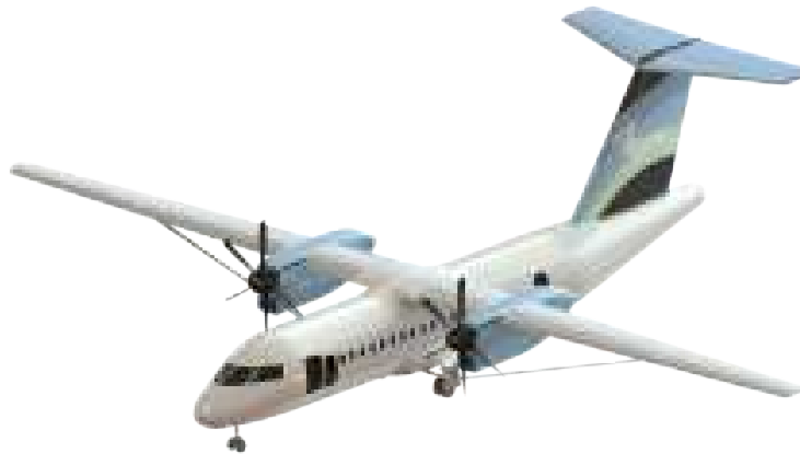
Fig. 10 Final Configuration with Truss-Braced Wing
